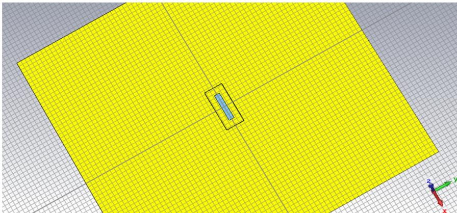
Figure 6.1: Slot antenna fed by a WR42 waveguide.
