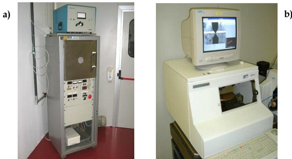
Fig. 2.12 – Tencor P-10 Surface Profiler (a) and Plasmafab 508 for oxygen plasma etching (b).
