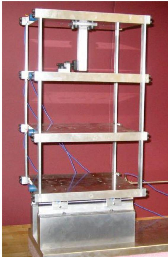
Figure 65. Test structure (Figueiredo, Park, Figueiras, Farrar, & Worden, 2009)
