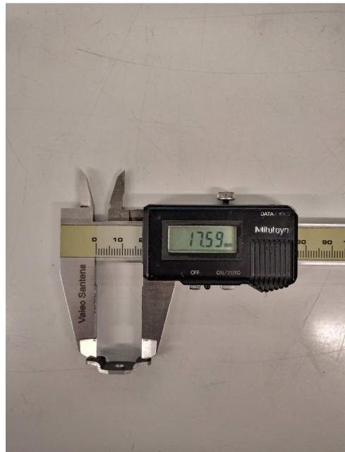
Figure 1.12 – Omega pad, lateral holes distance
