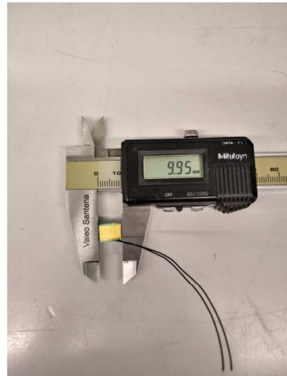
Figure 1.19 – Windings assembly, diameter.
