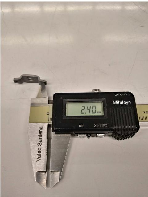
Figure 1.11 – Omega pad, lateral hole diameter
