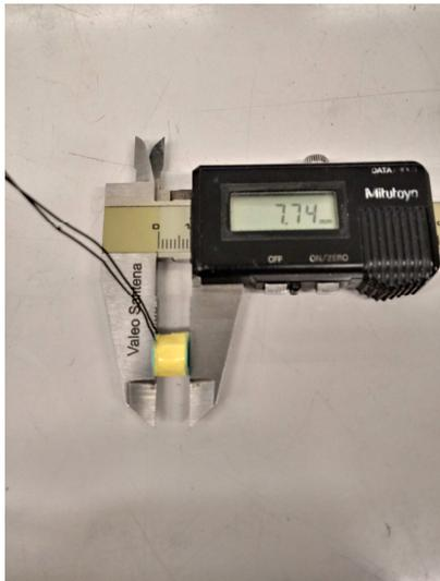
Figure 1.18 – Windings assembly, height.
