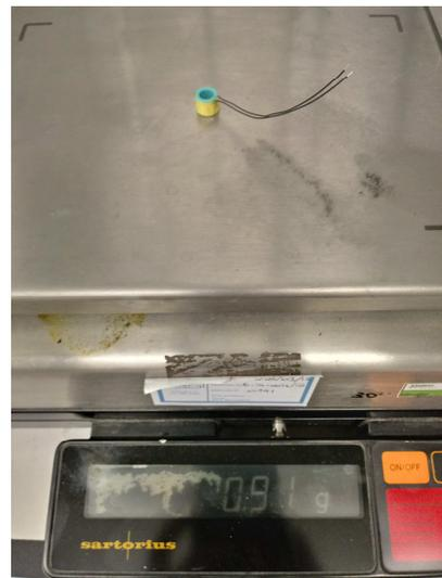
Figure 1.21 – Windings assembly with protective foil, mass measurement.
