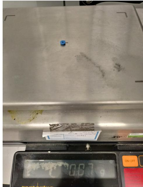
Figure 1.28 – Spacer, mass measurement.
