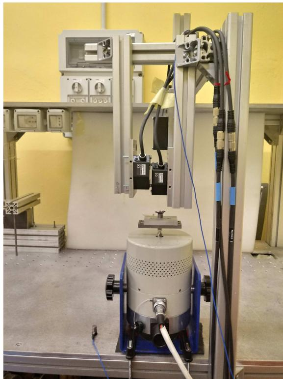
Figure 5.2 – Clamped free configuration.
