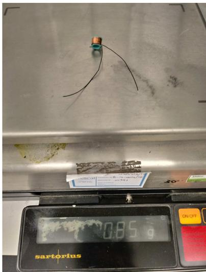
Figure 1.20 – Windings assembly, mass measurement.
