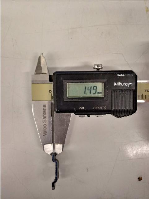
Figure 1.9 – Omega pad, thickness
