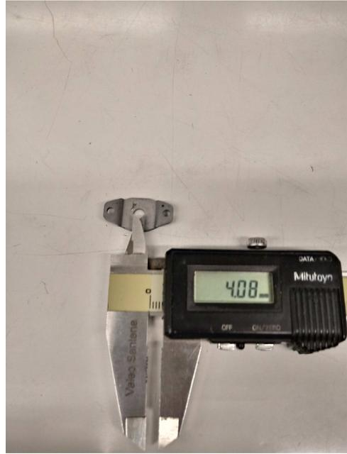
Figure 1.10 – Omega pad, main hole diameter
