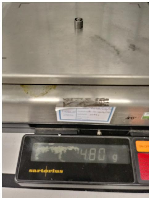
Figure 1.26 – Metallic body, mass measurement
