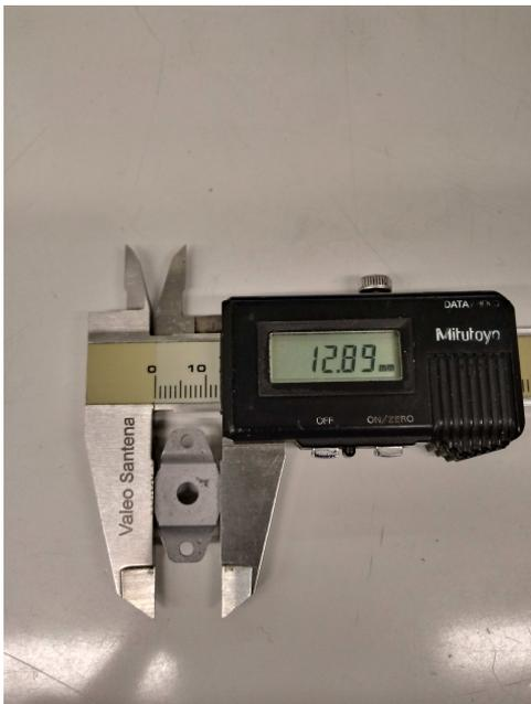
Figure 1.7 – Omega pad, width.
