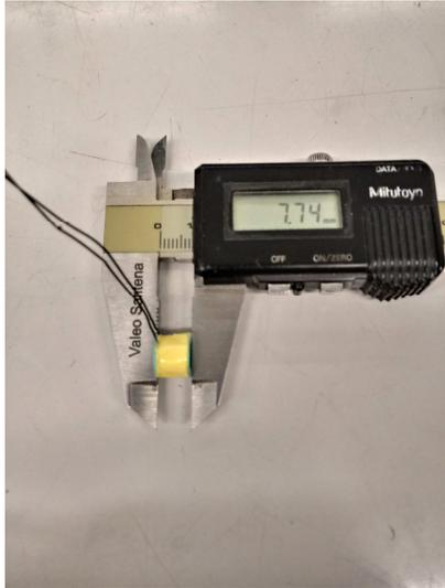
Figure 1.18 – Windings assembly, height.
