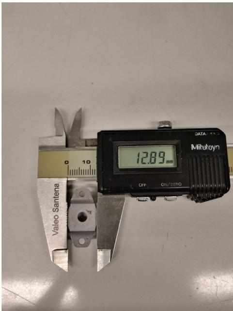
Figure 1.7 – Omega pad, width.
