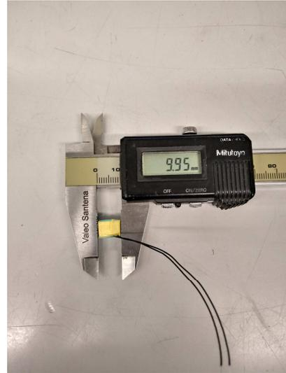
Figure 1.19 – Windings assembly, diameter.
