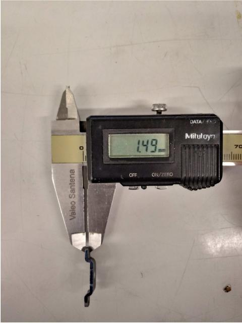
Figure 1.9 – Omega pad, thickness
