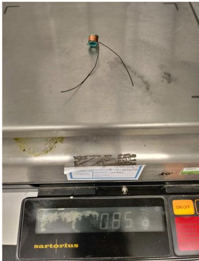
Figure 1.20 – Windings assembly, mass measurement.
