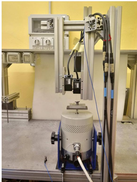
Figure 5.2 – Clamped free configuration.
