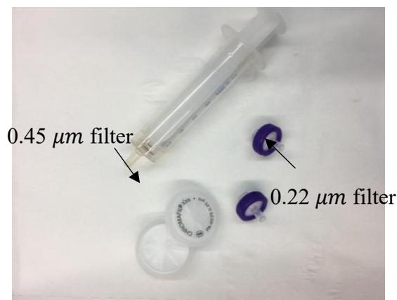
*Figure 31 - Syringe and the two types of filters*
