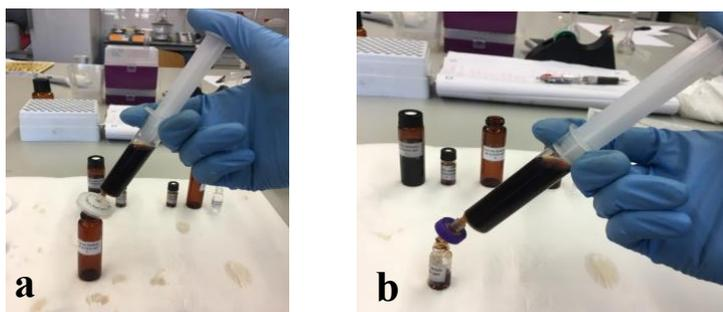
**Figure 32** - a) Filtration with a 0.45 µm filter b) Filtration with a 0.22 µm to proceed with HPLC analysis
