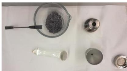
*Figure 28 - Homogenization of the mixture sample-diatomaceous earth and parts of the stainless-steel chamber*
