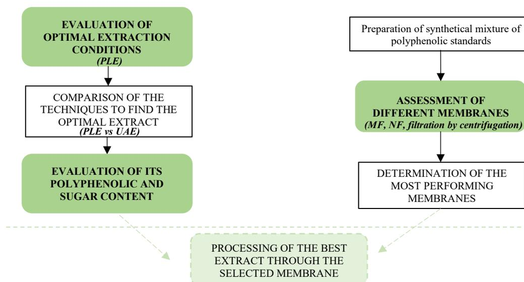
Figure 26 - General scheme of experimental methodology
