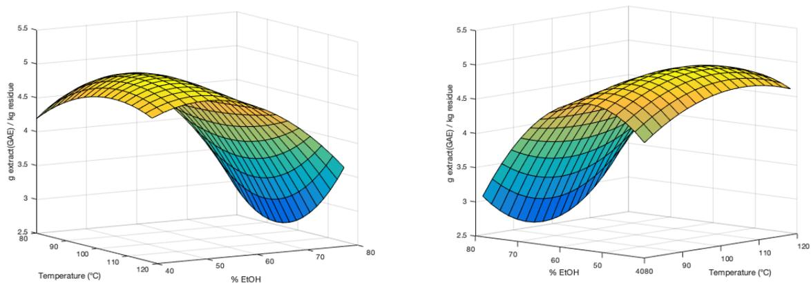
**Figure 40** - 3D surface representation of olive pomace PLE results
