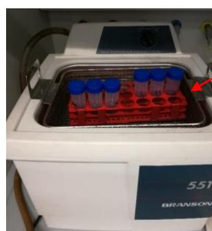
Distilled water ultrasonic bath with samples properly immersed
