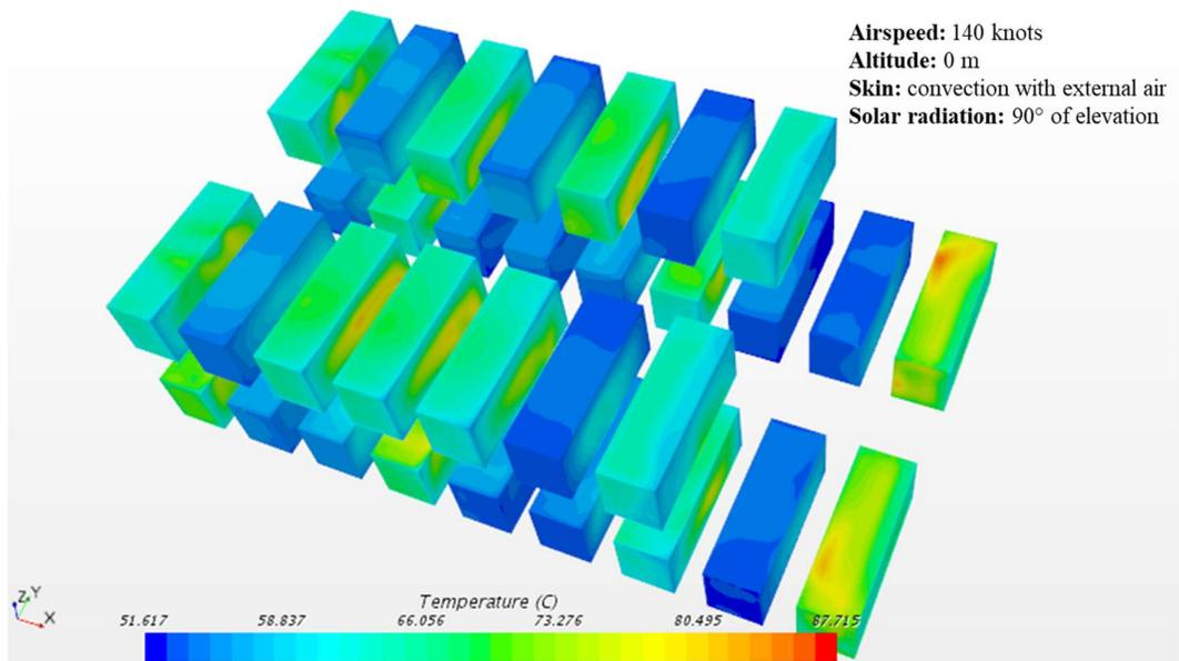
Figure 5.24: Test Case 3 - Internal Temperature - Upper View
