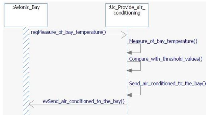
Figure 2.5: Provide Air Conditioning - Sequence Diagram 2
