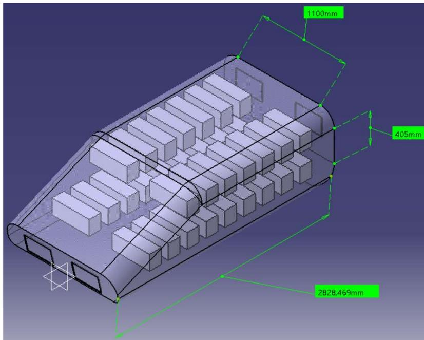
Figure 3.7: Avionic Bay CAD Model
