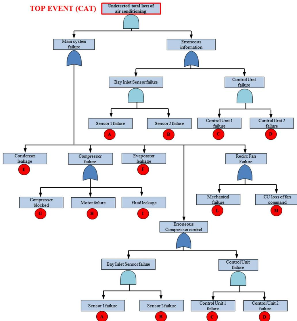
Figure 4.9: FTA - Vapour Cycle: *Undetected total loss of air conditioning*
