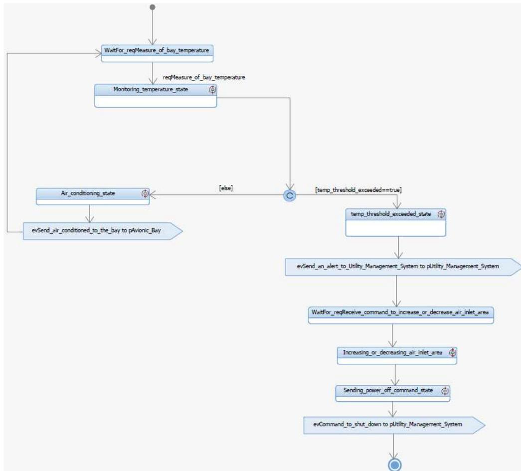
Figure 2.7: Provide Air Conditioning - State Machine Diagram
