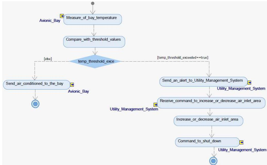
Figure 2.3: Provide Air Conditioning – Activity Diagram
