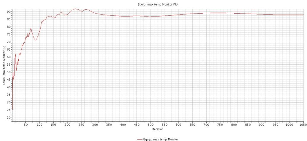
Figure 5.10: Maximum temperature of the most heated LRU
