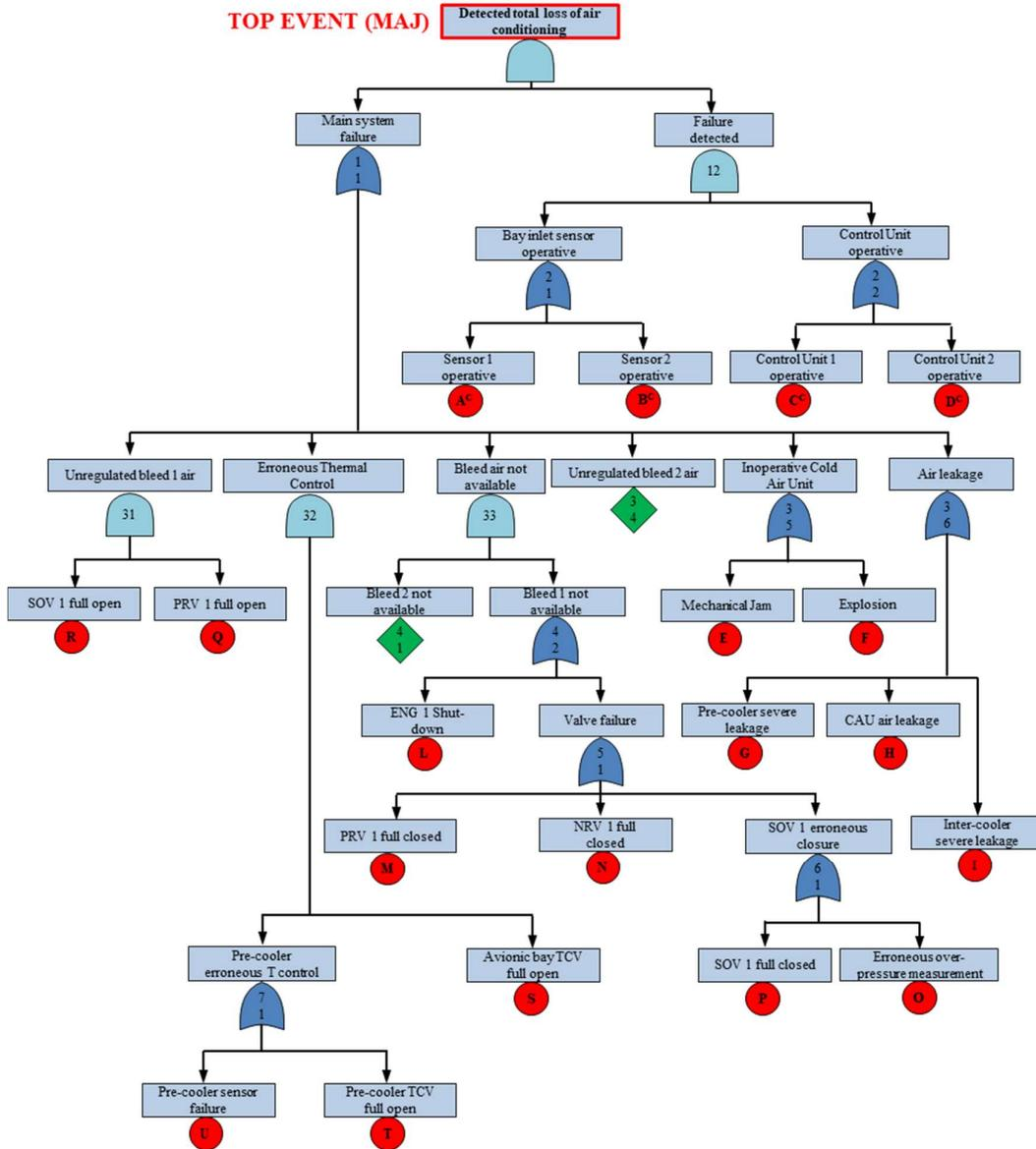
Figure 4.8: FTA - Air Cycle: *Detected total loss of air conditioning*
