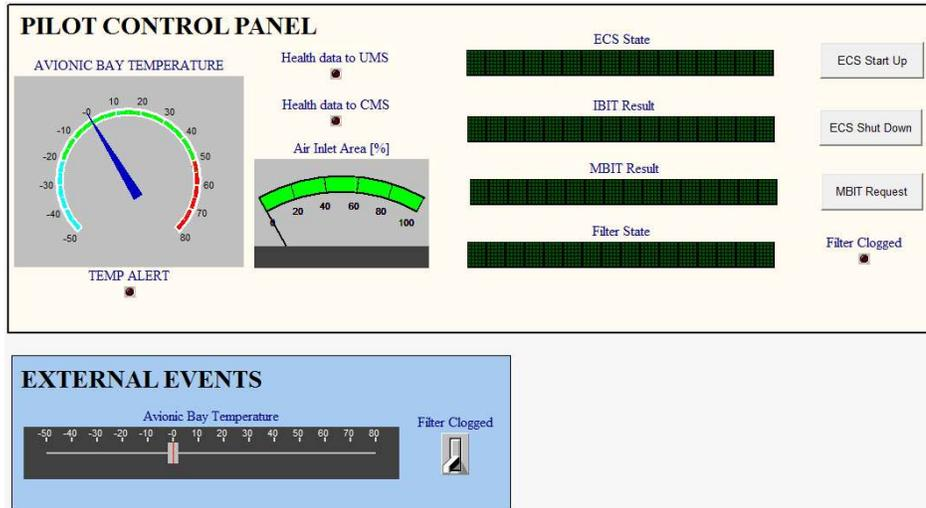
Figure 2.8: ECS Panel (Functional Model)
