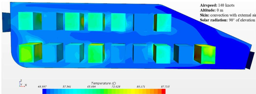
Figure 5.26: Test Case 3 - Internal Temperature - Lateral View
