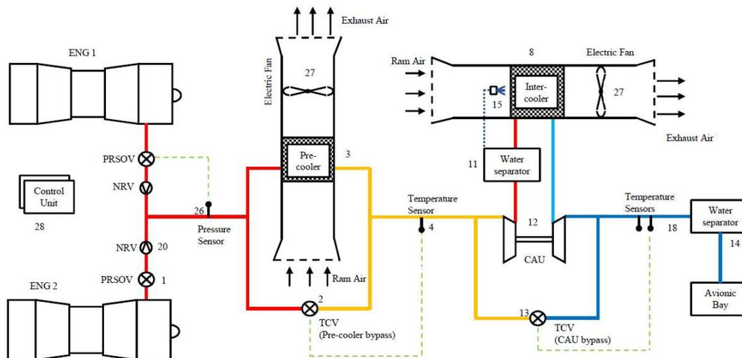
Figure 3.19: Air Cycle System Architecture
