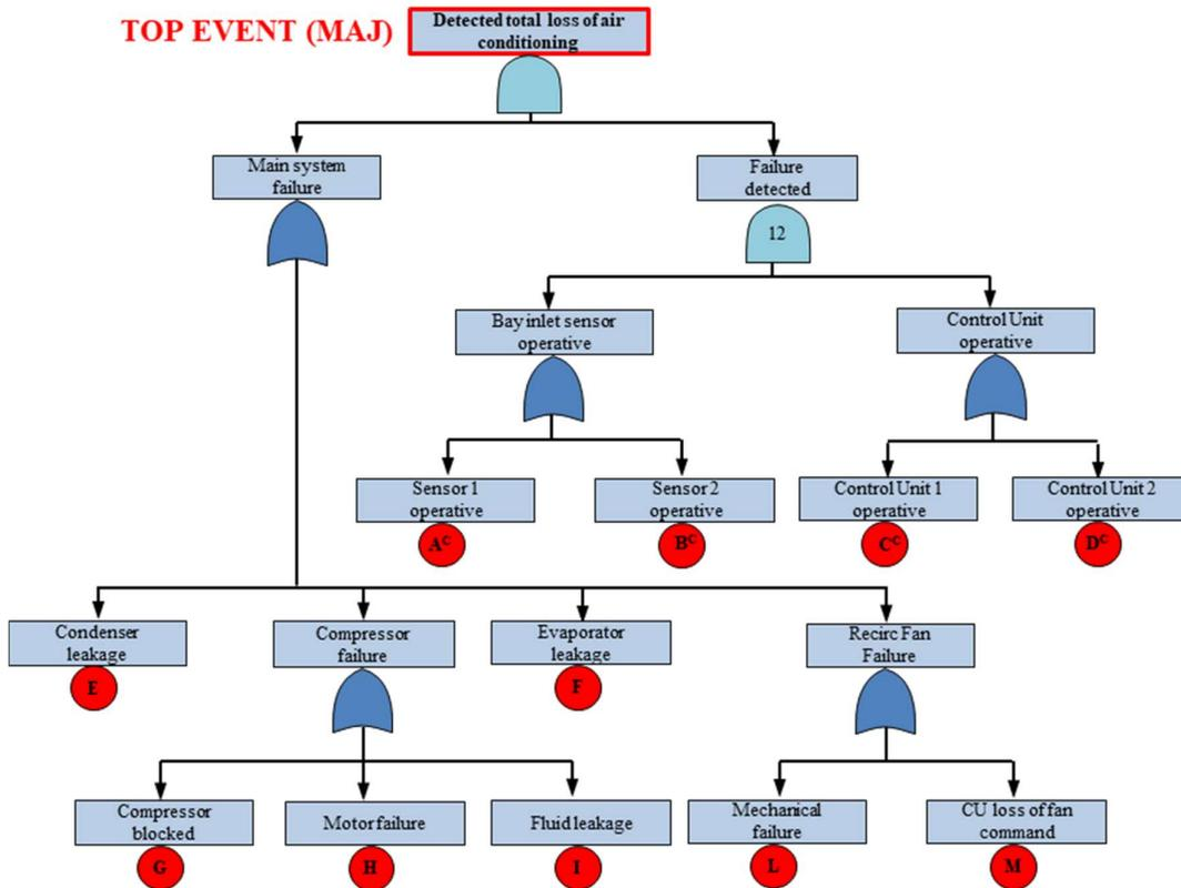
Figure 4.10: FTA - Vapour Cycle: *Detected total loss of air conditioning*
