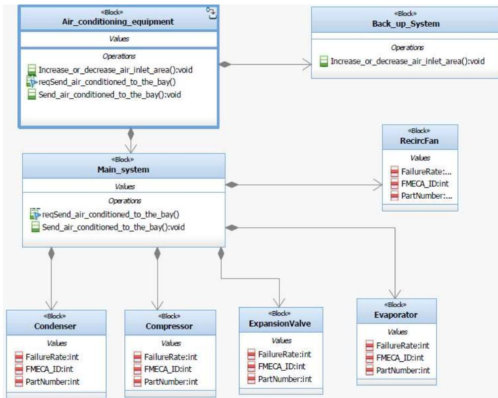
Figure 4.14: VCCS Block Definition Diagram
