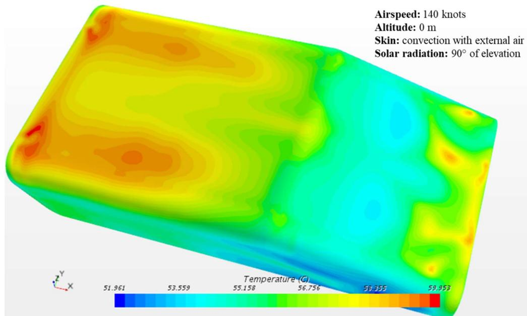
Figure 5.19: Test Case 3 - External Temperature
