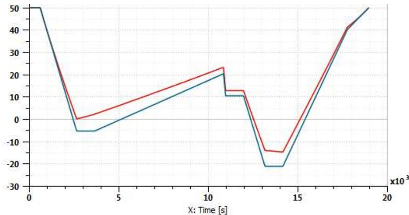
Figure 3.4: External and Recovery Temperatures [°C] – ISA+35
