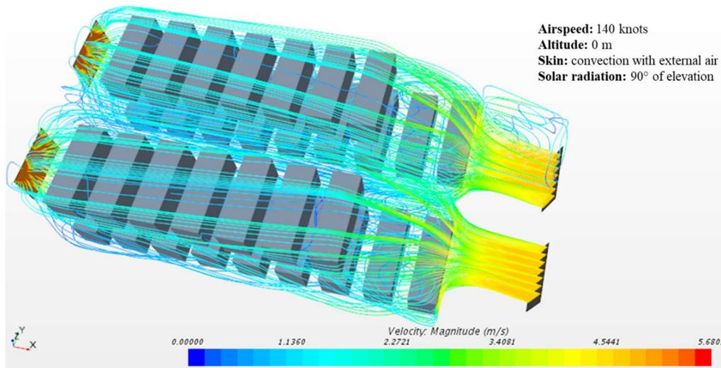
Figure 5.21: Test Case 3 - Velocity Streamlines
