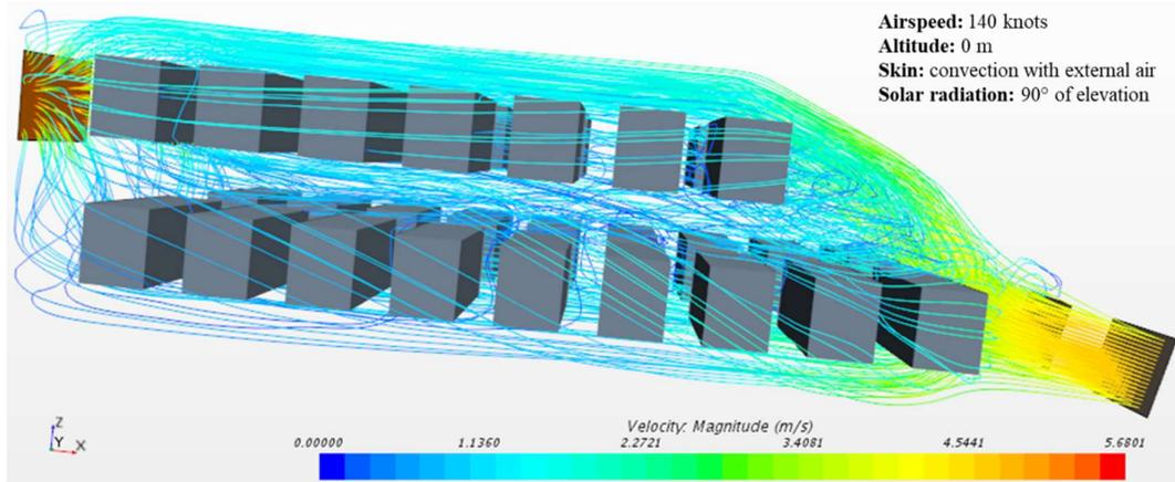
Figure 5.22: Test Case 3 - Velocity Streamlines - Lateral View
