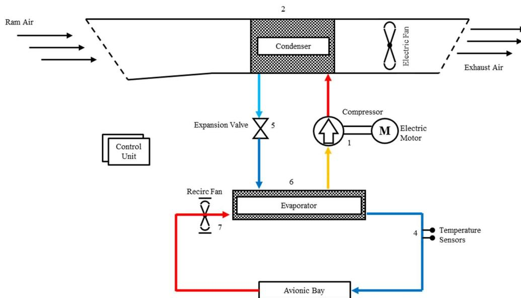
Figure 3.9: Vapour Cycle System Architecture
