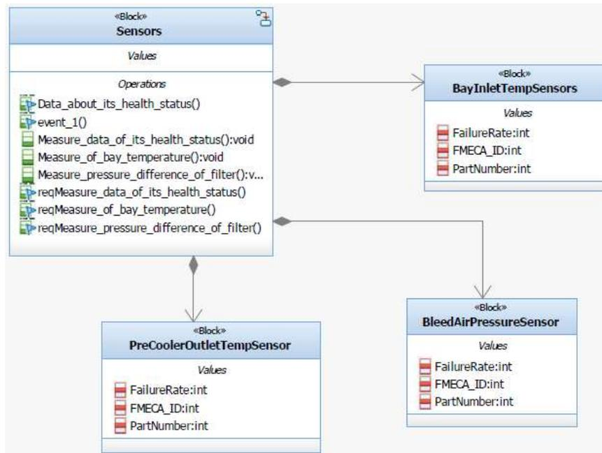
Figure 4.13: ACM Sensors Block Definition Diagram
