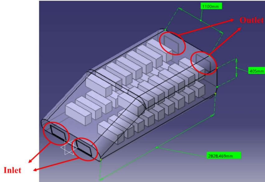
Figure 5.2: Avionic Bay CAD model
