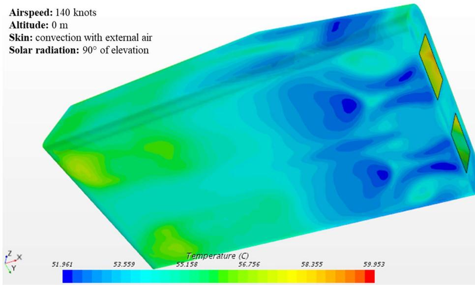
Figure 5.20: Test Case 3 - External Temperature - Inferior View
