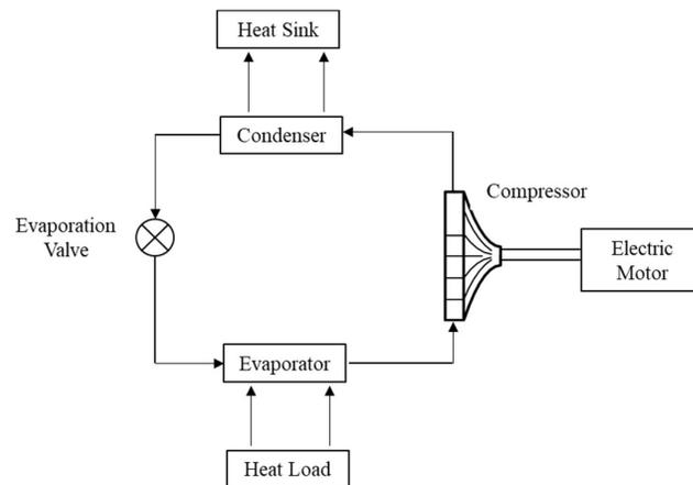
Figure 1.8: Vapour Cycle System (ref. [3])
