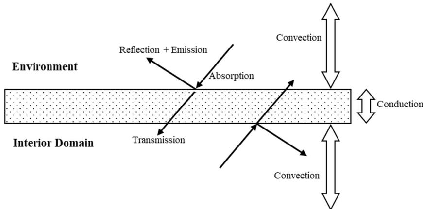
Figure 5.4: Heat Transfer Scheme (ref [11])
