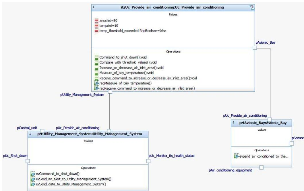
Figure 2.6: Provide Air Conditioning - Internal Block Diagram
