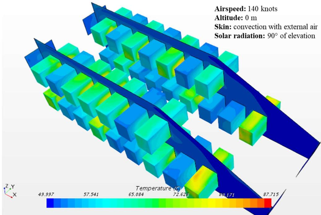
Figure 5.25: Test Case 3 - Internal Temperature
