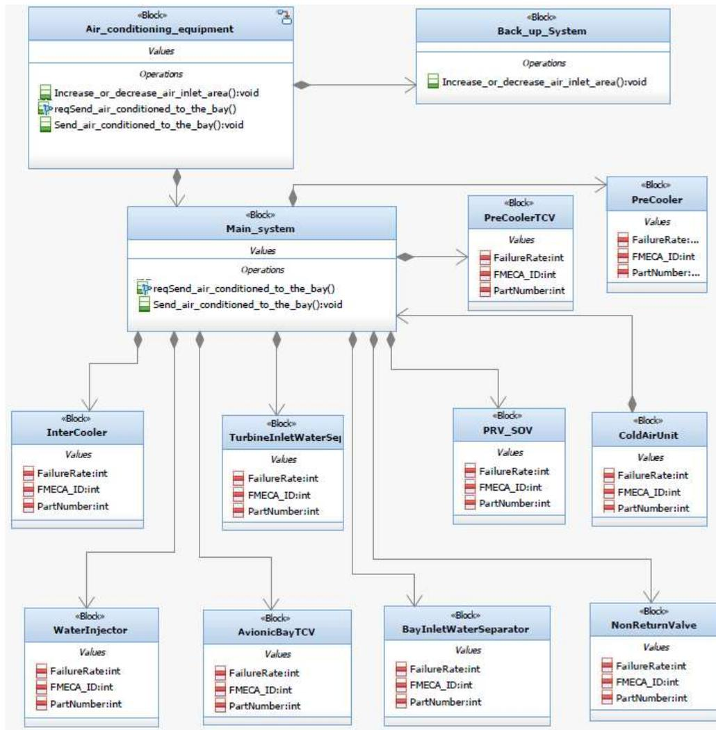
Figure 4.12: ACM Block Definition Diagram
