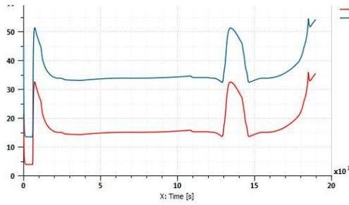
Figure 3.11: Inlet and Outlet Bay Temperature
