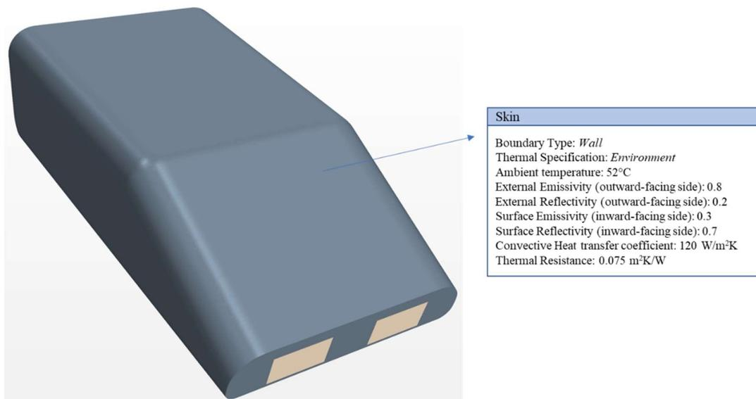
Figure 5.14: Boundary Specification - External View
