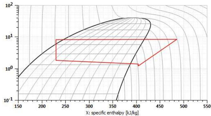
Figure 3.8: Vapour Cycle diagram (Specific Enthalpy [kJ/kg] - Pressure [bar])
