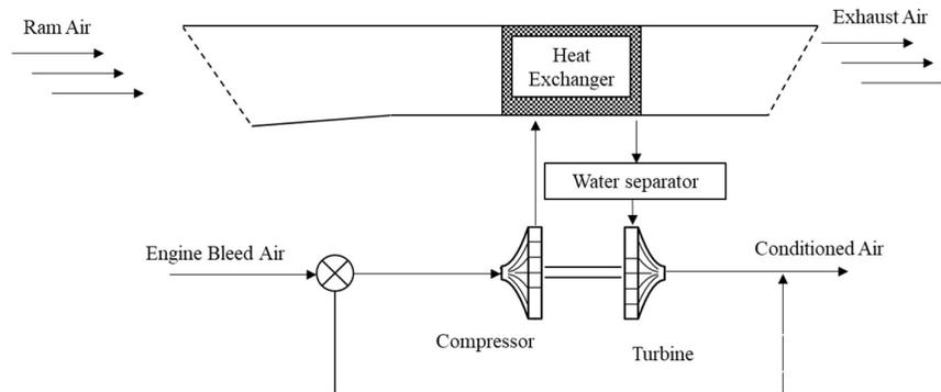
Figure 1.7: Air Cycle System (ref. [3])
