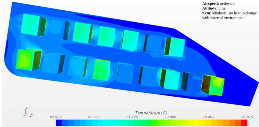
Figure 5.12: Test Case 1 - Internal Temperature - Lateral View
