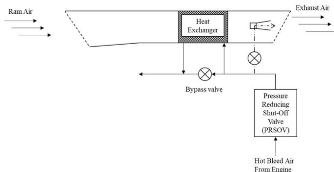
Figure 1.6: Bleed Air Thermal Control (ref. [3])
