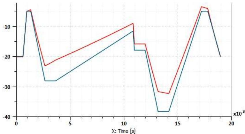
Figure 3.5: External and Recovery Temperatures [°C] – ISA-35
