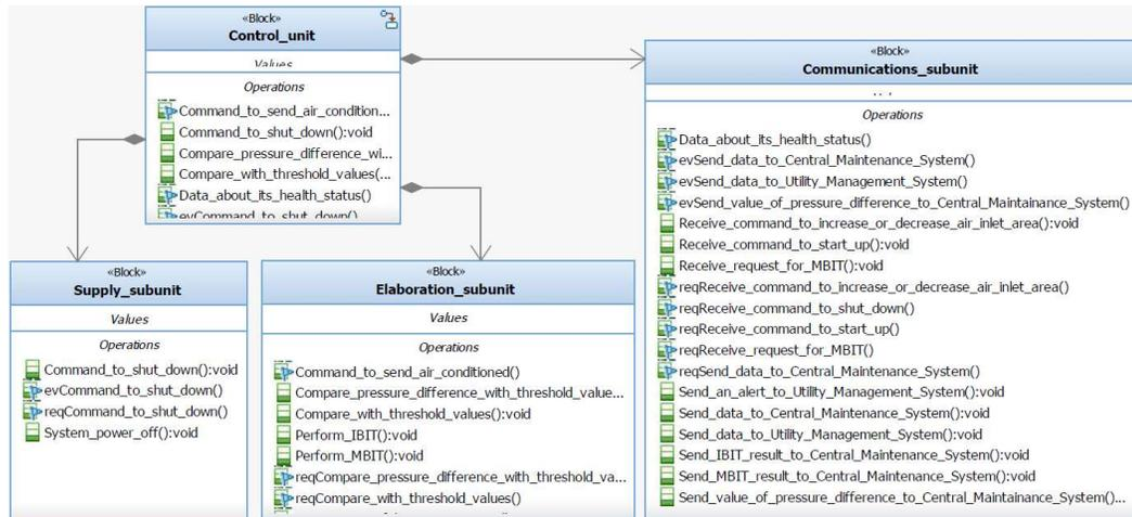
Figure 4.11: Control Unit Block Definition Diagram
