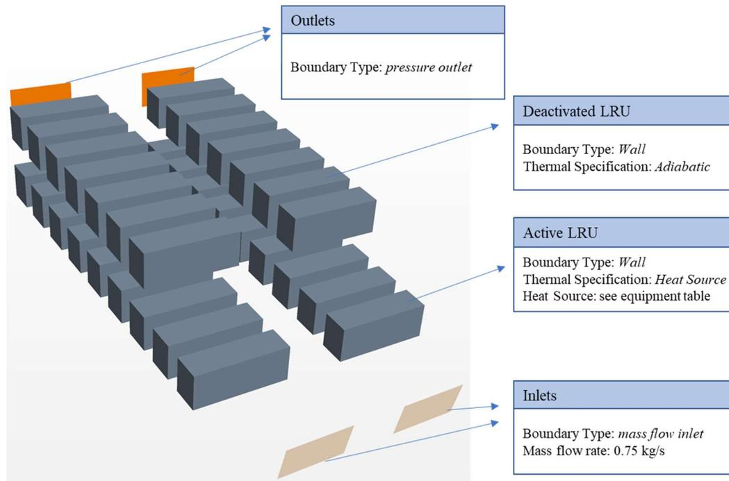
Figure 5.8: Boundary Specifications - Internal View
