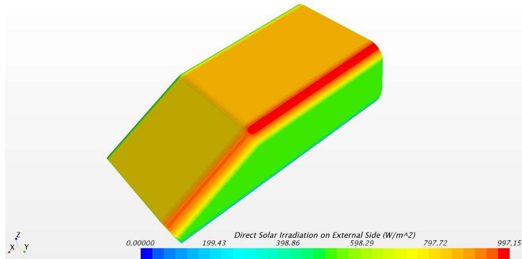
Figure 5.17: Direct Solar Irradiation,  $60^\circ$
