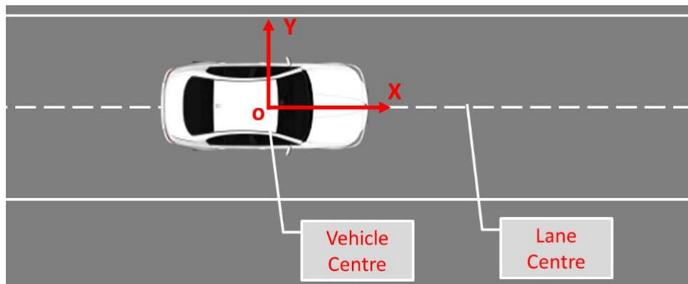
Figure 2-7 Lateral offset (LO), coordinate system
