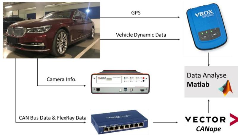
Figure 2-1 The driving behavior collection system
