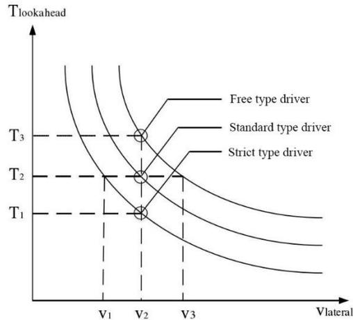
Figure 3-6 Schematic diagram of FOD algorithm with different types drivers
