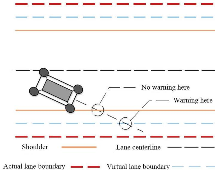
Figure 3-5 Schematic diagram of FOD algorithm
