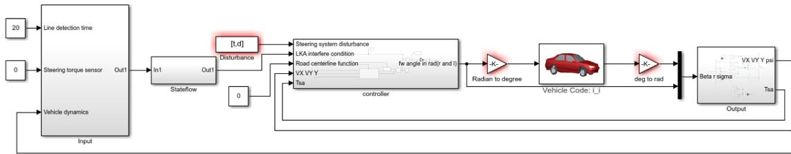
Figure 5-9 CarSim S-Function in loop
