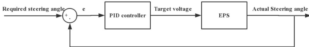
Figure 5-3 Control block of EPS controller
