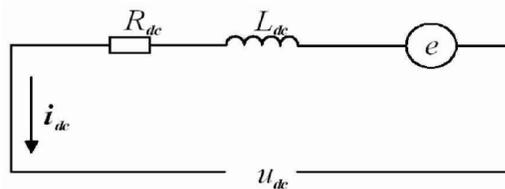
Figure 5-2 Equivalent circuit of DC brush motor
