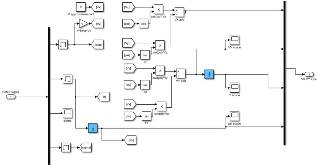
Figure 5-4 Converting  $V_x, V_y$  into  $V_X, V_Y$
