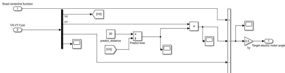
Figure 5-5 Path error controller
