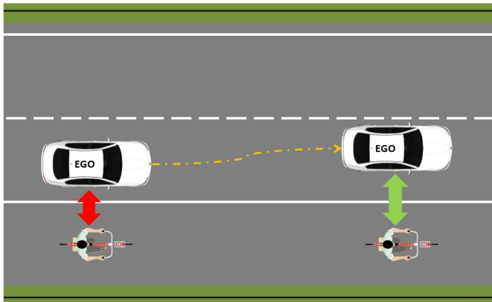
Figure 1-6 Adaptive adjustment of lane keeping based on driving conditions
