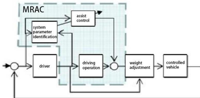
Figure 1-4 The Variable Structure-Model Reference Adaptive Controller (VS-MRAC)
