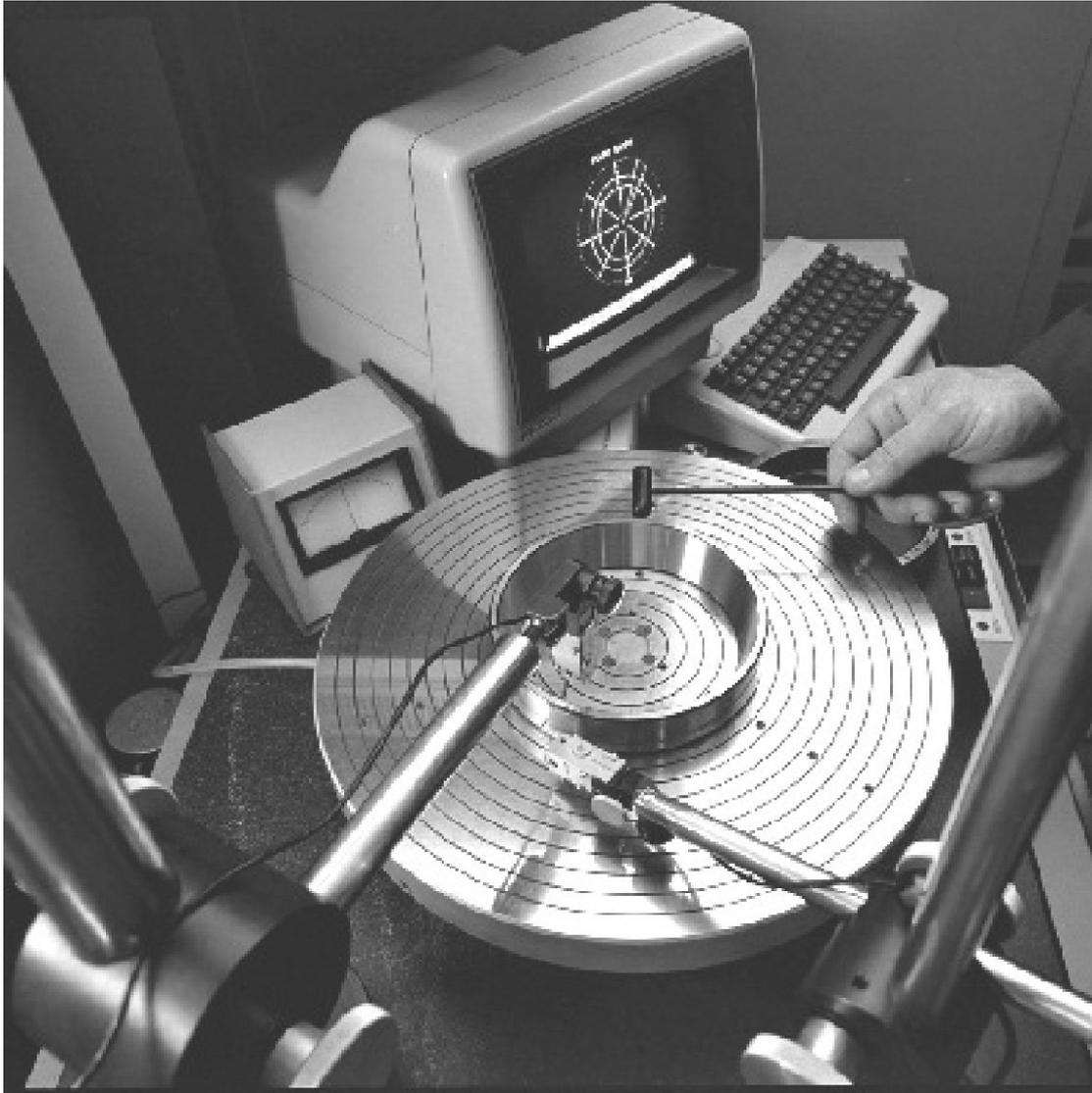
FIGURE 7.8 Bearing component waviness tester. (Courtesy of Timken Company.) from [1]
