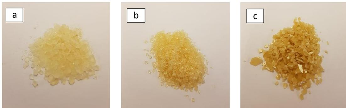
Fig. 9. In the first picture (a) low reactivity particles, in (b) the medium and in (c) the high.
