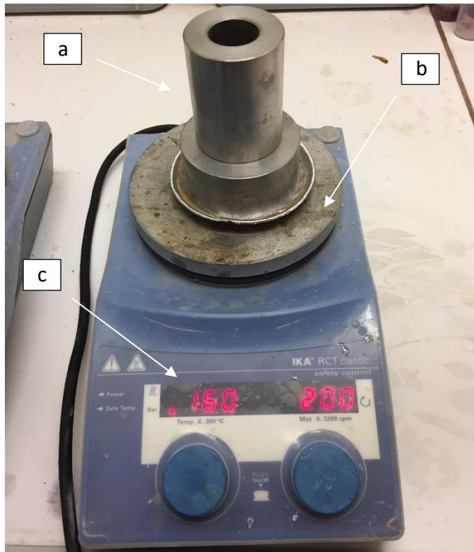
Fig. 11. Preparation of healing agent layer for bond strength test; the constant pressure is applied through the cylindrical mass (a) on the top of the heating plate (b). In (c) the indicator of temperature in degree Celsius.
