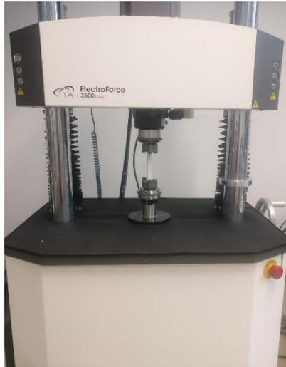
Figure 26. ElectroForce 3500 series Universal testing machine
