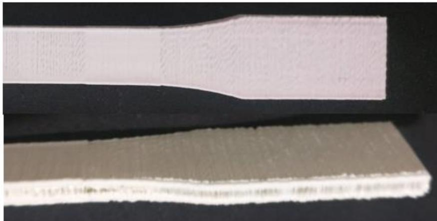
Figure 30. Defects of vertical printed component: on the top, different in the filament deposition; on the bottom, contour problems
