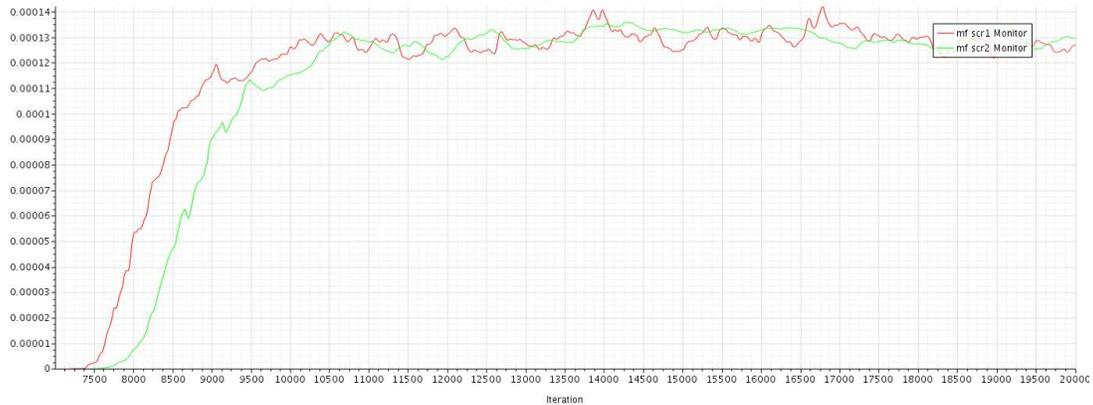
**Figure 11.1** Mass fraction H2O computed on SCR section. Red SCR1, green SCR2.
