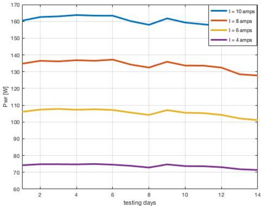
Figure 31 Comparison between power distributions at different values of current
