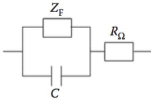
Figure 19 Common equivalent circuit describing the frequency response of a fuel cell
