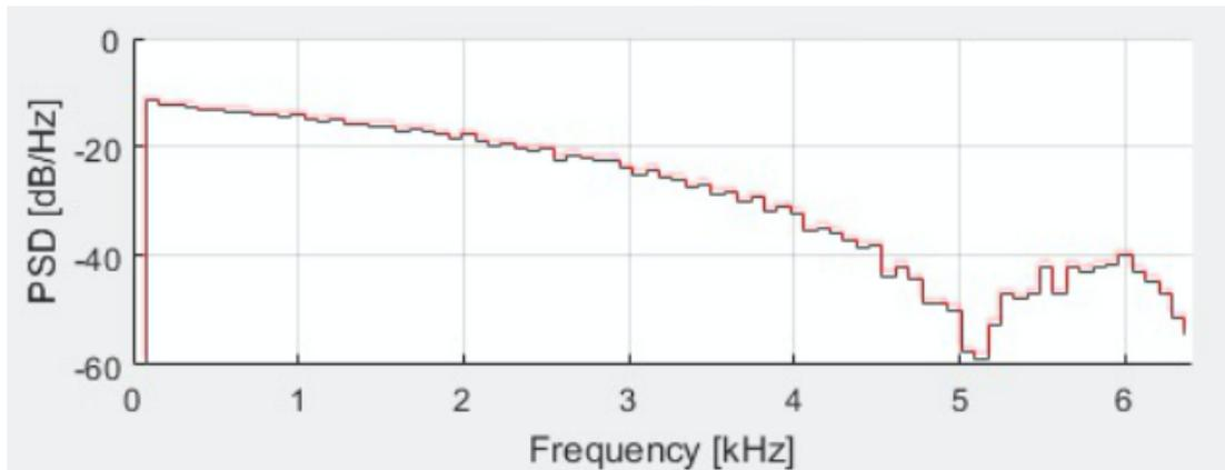
*Figure 6 Power Spectral Density of a PRBS signal*
