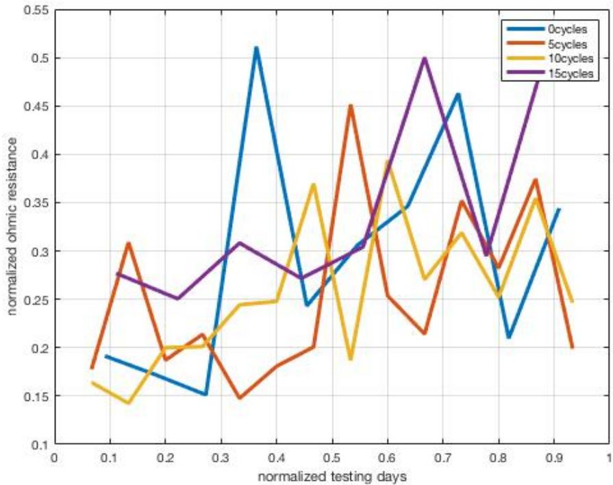
The plot shows the drastic fluctuations that characterized the behavior of the resistance, which is probably due to the fact that the efficiency of the ionic conduction does not only depend on the age of the fuel cell, or in how much time the cell has been working even though it is a fact that the resistance got higher at the end of the life of the fuel cell, especially as far as the resistance after 15 cycles is concerned.
