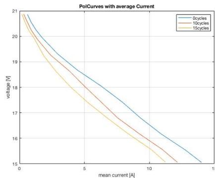
Figure 13 Polarization Curves referring to the 7th day of testing (25 March)
