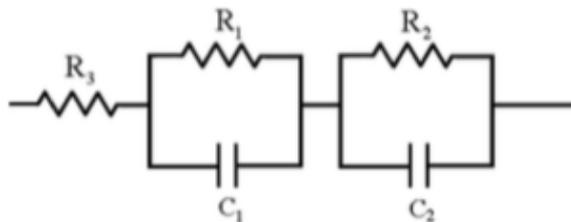
Figure 22 Equivalent circuit proposed by Niya et al. in their EIS review for the Journal of Power Sources 240(2013)281-293
