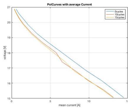
Figure 12 Polarization Curves Referring to the 5<sup>th</sup> day of testing (21st of March)
