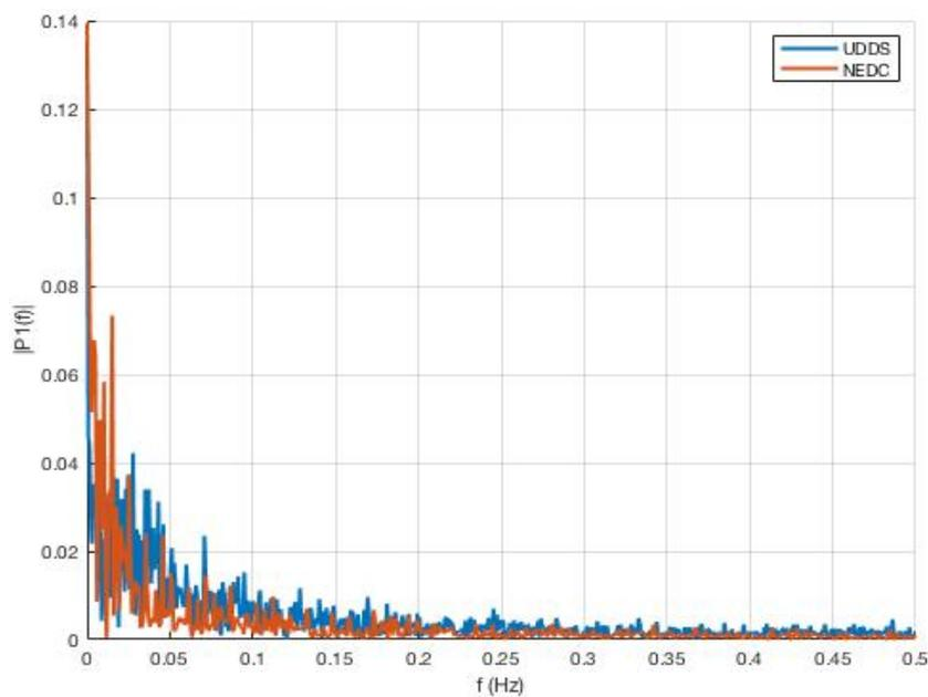
Figure 9 Comparison of the FFT of the power profile of UDDS and NEDC cycle
