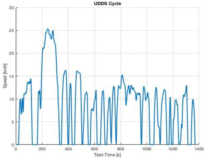
Figure 7 Speed Profile of the UDDS cycle
