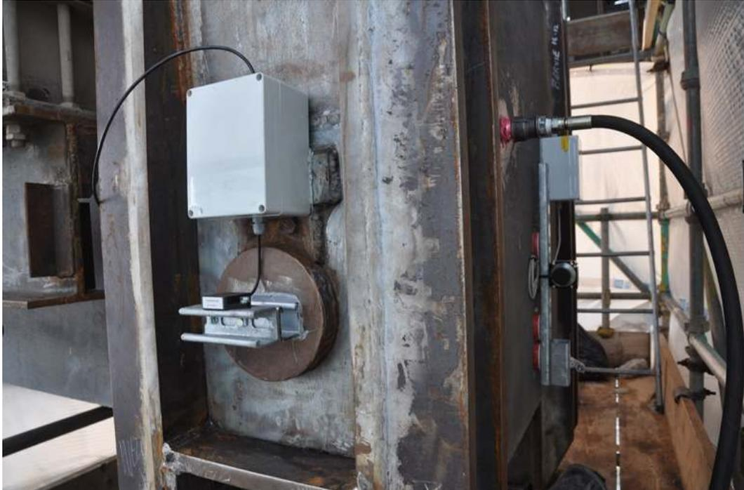
*Figure 4.10: Tiltmeter on truss end link NEMS (Kitching, 2017)*
