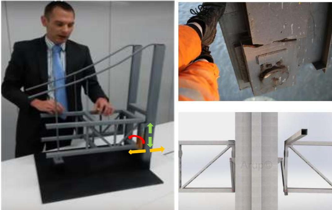
Figure 3.4: End truss link movement diagram and fracture photos (Arndt,2015)
