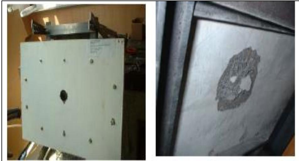
**Figure4. 4:** impact resistance of Ferro-cement sample
