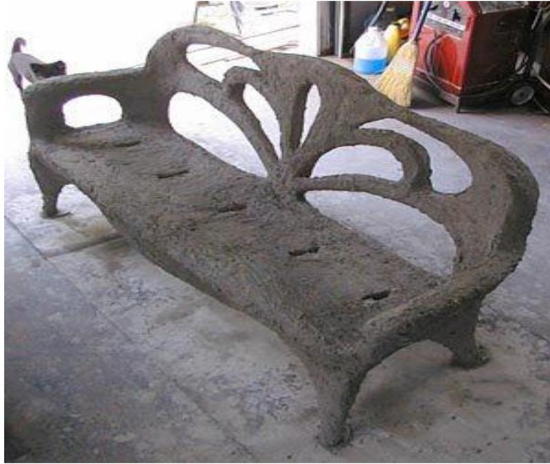
**Figure5. 18:** Ferro-cement Bench
