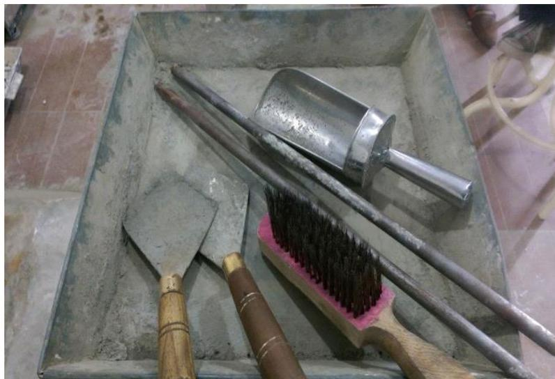
**Figure3. 11**Trowels, trays and tamping rods
