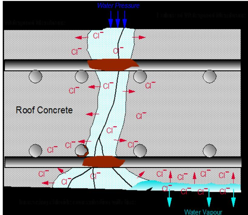
**Figure4. 3:** Chloride diffusion due to salt water
