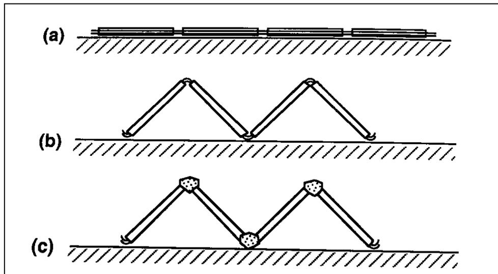
**Figure5. 6:** Typical production of Ferro-cement W-shaped elements from Flat sheet (NAMAAN 2000)
