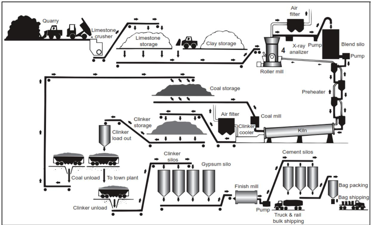
**Figure3. 6:** Flow diagram of the dry process for Portland cement manufacture (Mehta & Monteiro, 2006)
