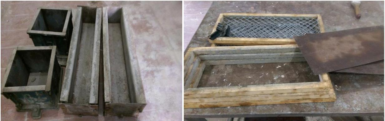
**Figure3. 10:** Different sizes of Moulds, cubes and panels
