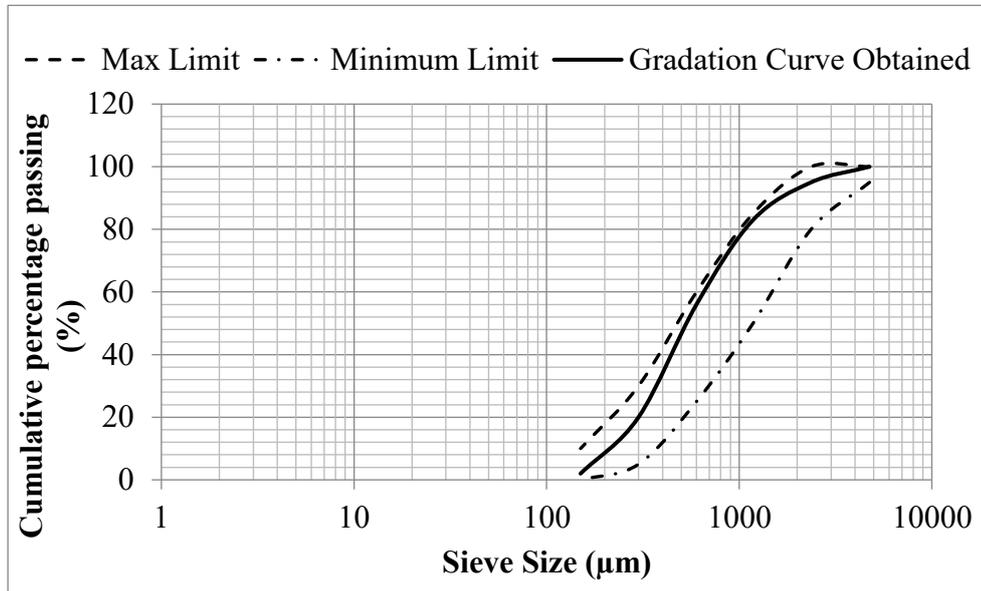
**Figure3. 8:** Gradation curve for sand
