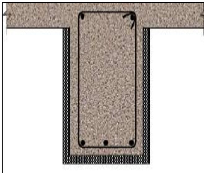
**Figure4. 5:** Section of T beam is platted with Ferro-cement
