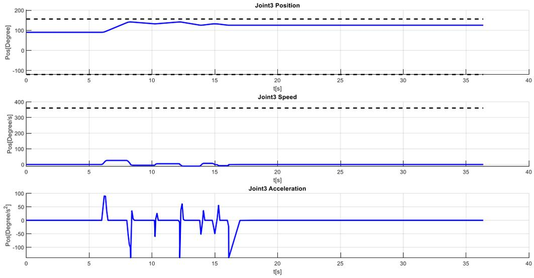
Figure 0-16 KR6 r700: Joint 3 – position, speed and acceleration profiles
