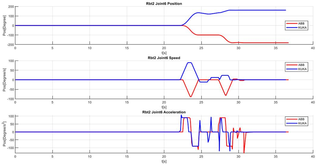
Figure 0-37 IRB1600 vs KR10 r1100: Joint 6 – position, speed and acceleration profiles
