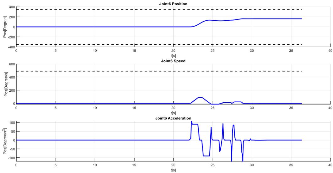
Figure 0-25 KR10 r1100: Joint 6 – position, speed and acceleration profiles
