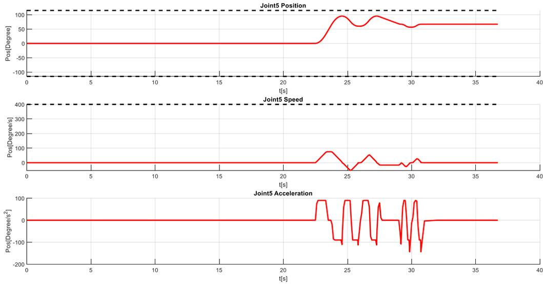
Figure 0-12 IRB 1600: Joint 5 – position, speed and acceleration profiles
