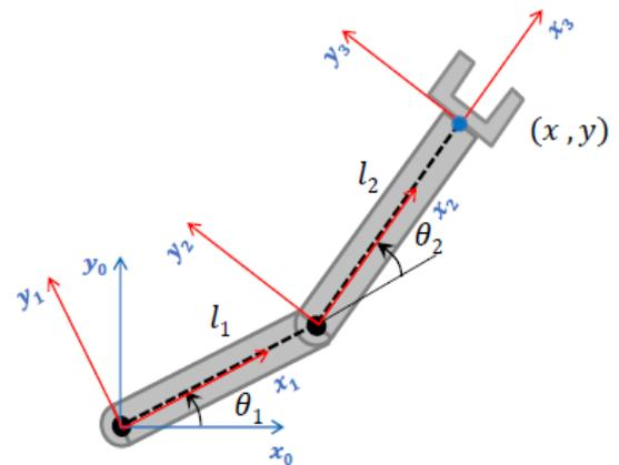
Figure 0-2 Forward kinematics model
