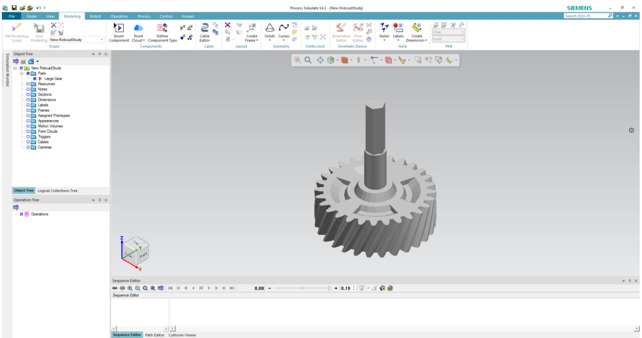
Figure 0-17 The large gear Process Simulate model
