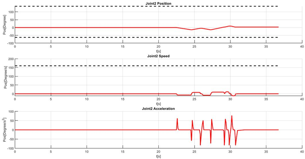
Figure 0-9 IRB 1600: Joint 2 – position, speed and acceleration profiles
