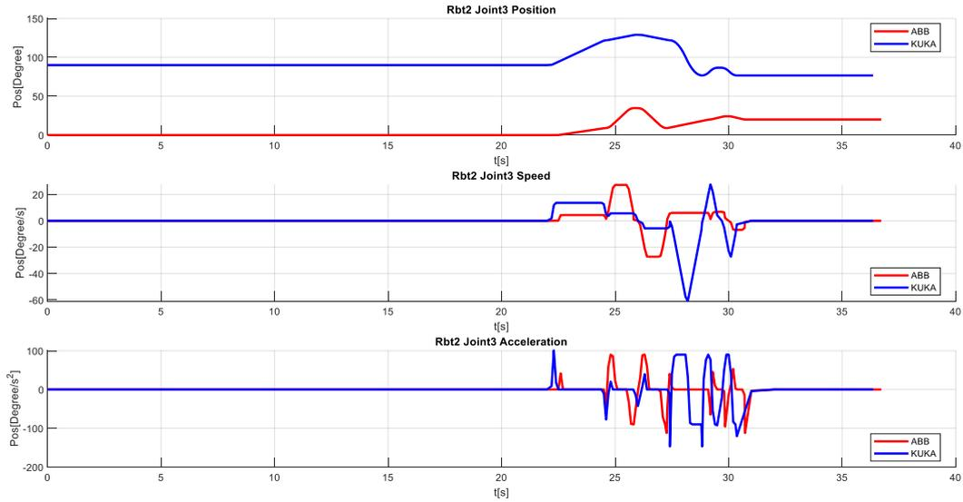
Figure 0-34 IRB1600 vs KR10 r1100: Joint 3 – position, speed and acceleration profiles
