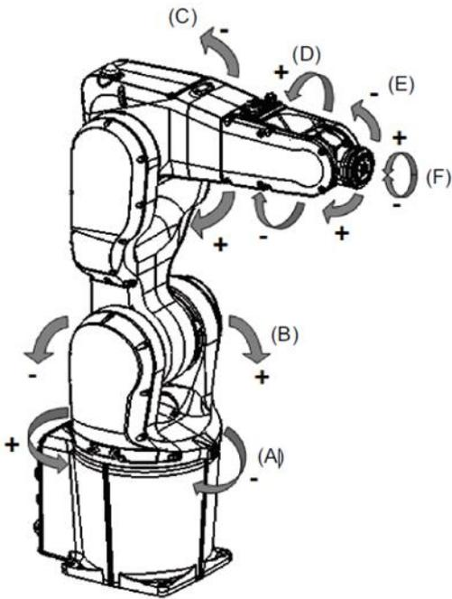
Figure 0-2 Manipulator axes
