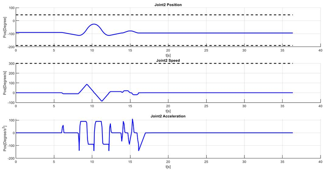
Figure 0-15 KR6 r700: Joint 2 – position, speed and acceleration profiles
