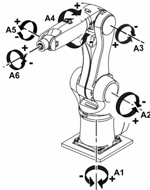
Figure 0-10 Manipulator axes
