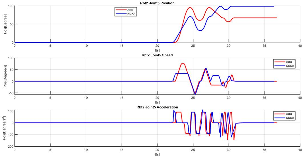
Figure 0-36 IRB1600 vs KR10 r1100: Joint 5 – position, speed and acceleration profiles
