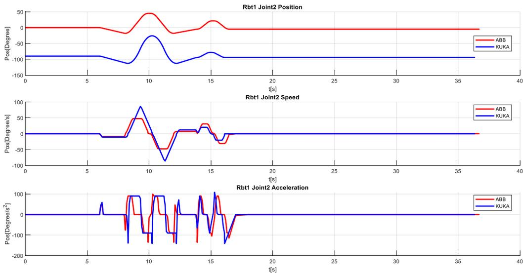
Figure 0-27 IRB1200 vs KR6 r700: Joint 2 – position, speed and acceleration profiles
