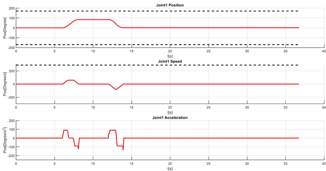
Figure 0-2 IRB 1200: Joint 1 – position, speed and acceleration profiles
