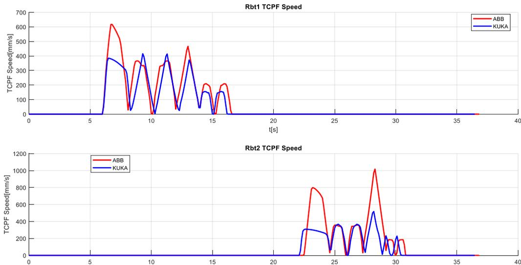
Figure 0-38 IRB1200 vs KR6 r700 and IRB1600 vs KR10 r1100 – TCPF speed profiles
