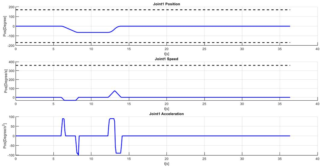
Figure 0-14 KR6 r700: Joint 1 – position, speed and acceleration profiles
