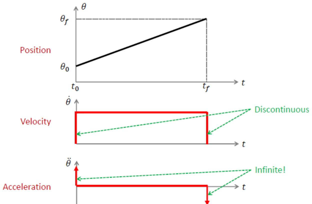
Figure 0-1 Linear joint interpolated motion
