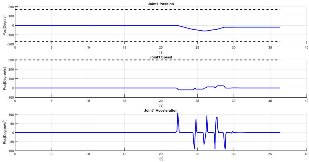
Figure 0-20 KR10 r1100: Joint 1 – position, speed and acceleration profiles
