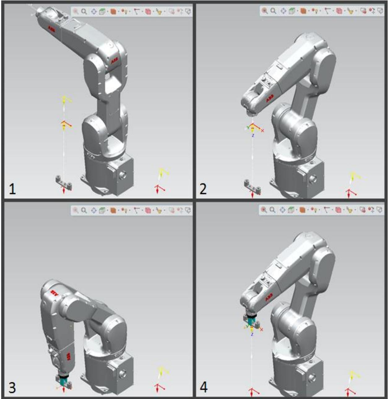
Figure 0-5 IRB 1200 pick poses: 1 home, 2 via (approach) location, 3 pick location, 4 via (retract) location
