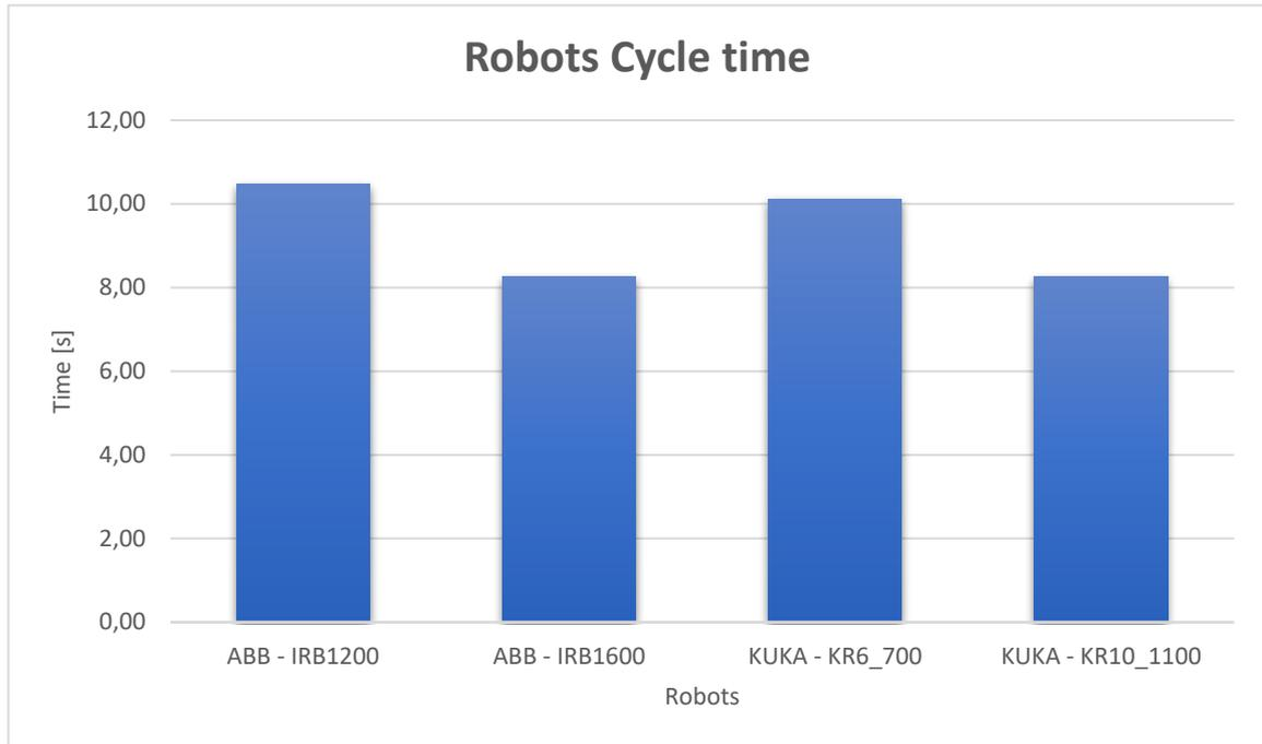
Figure 0-41 Robots cycle time
