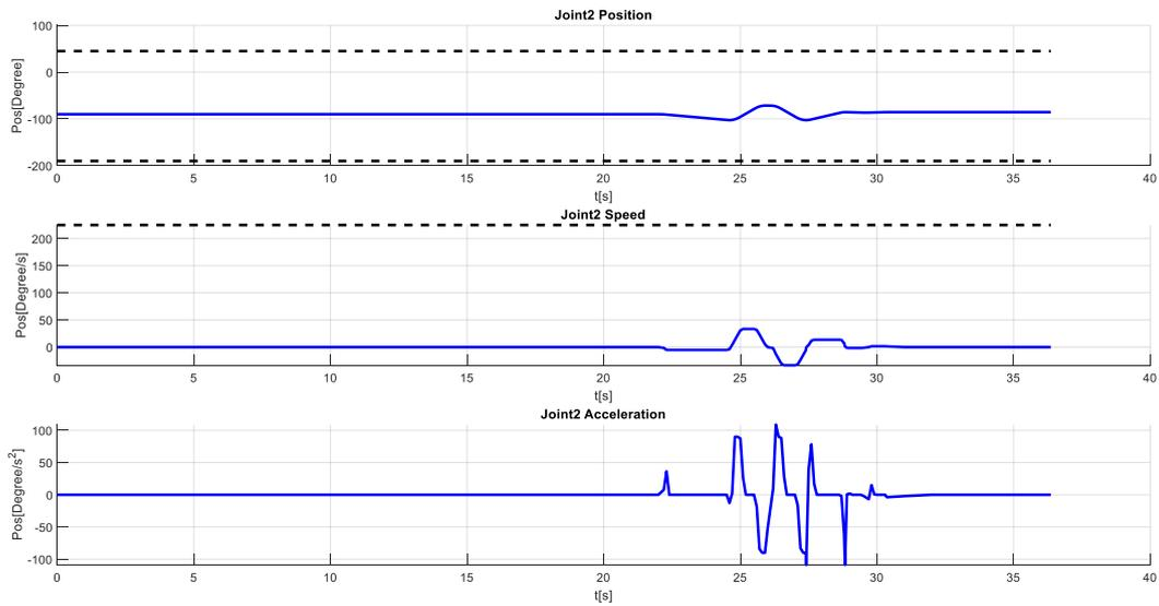
Figure 0-21 KR10 r1100: Joint 2 – position, speed and acceleration profiles
