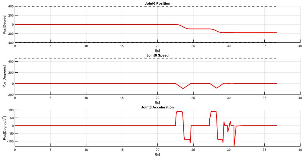
Figure 0-13 IRB 1600: Joint 6 – position, speed and acceleration profiles
