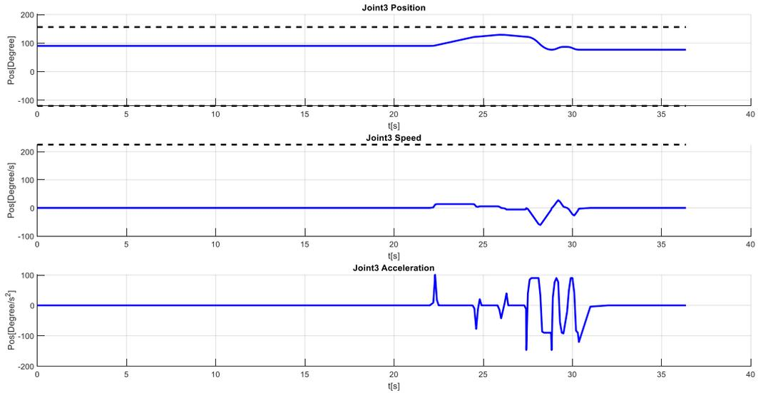
Figure 0-22 KR10 r1100: Joint 3 – position, speed and acceleration profiles
