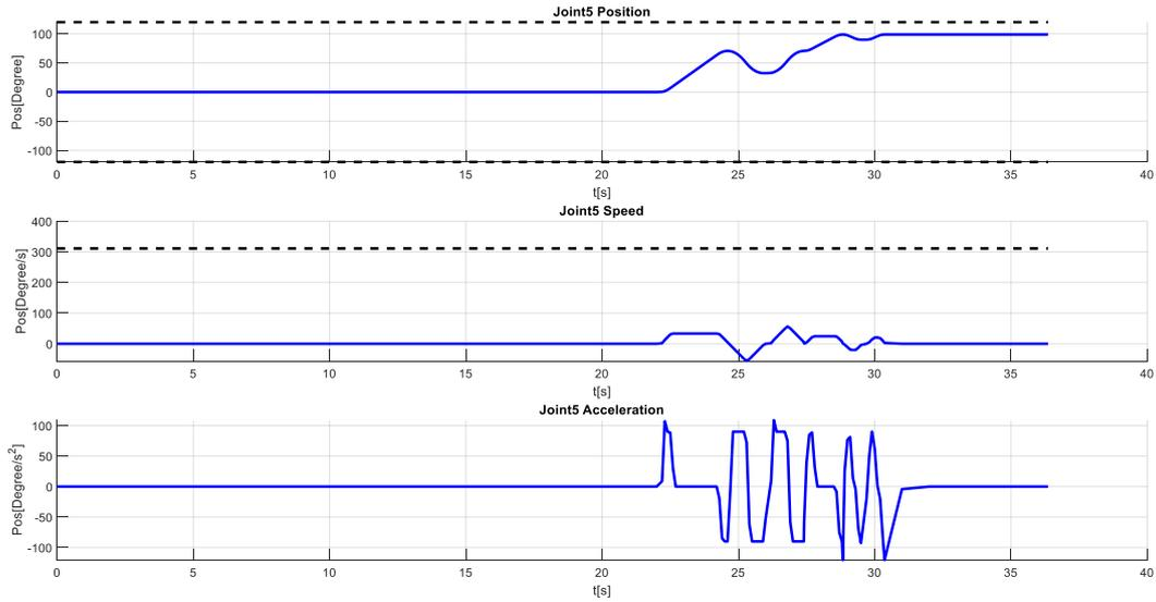
Figure 0-24 KR10 r1100: Joint 5 – position, speed and acceleration profiles
