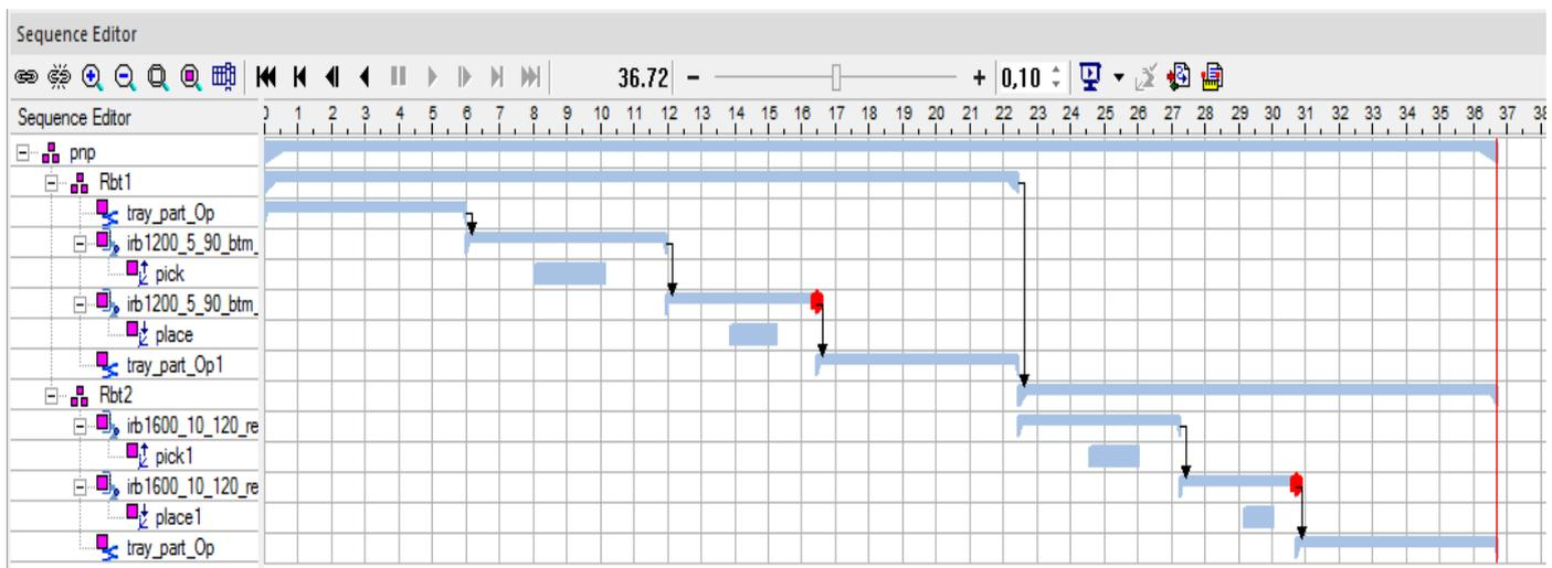
Figure 0-2 ABB sequence editor after simulation
