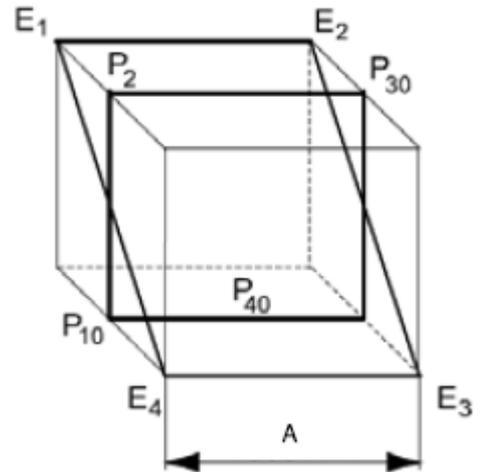
Figure 0-7 Working space with  $A = 400$  mm
