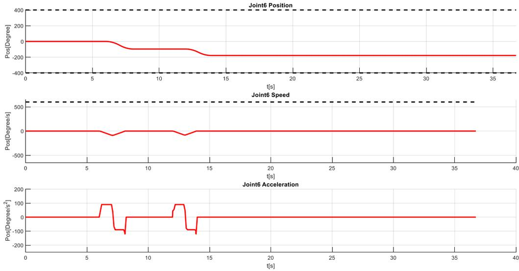
Figure 0-7 IRB 1200: Joint 6 – position, speed and acceleration profiles
