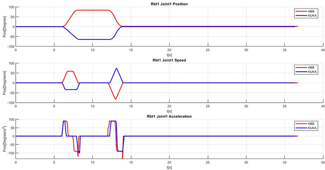
Figure 0-26 IRB1200 vs KR6 r700: Joint 1 – position, speed and acceleration profiles
