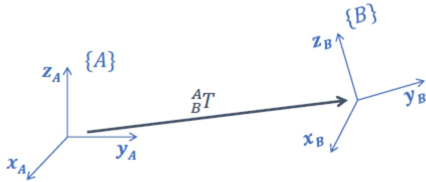
Figure 0-3 Assigning frames to links idea
