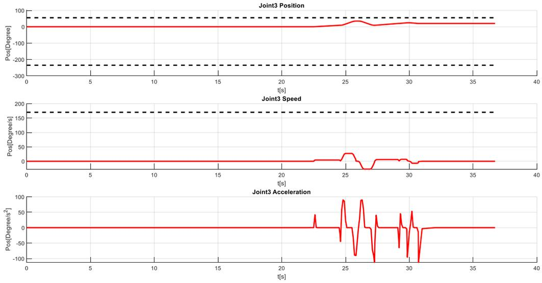
Figure 0-10 IRB 1600: Joint 3 – position, speed and acceleration profiles
