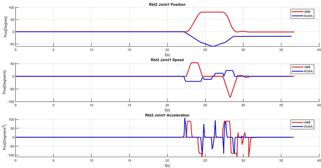
Figure 0-32 IRB1600 vs KR10 r1100: Joint 1 – position, speed and acceleration profiles
