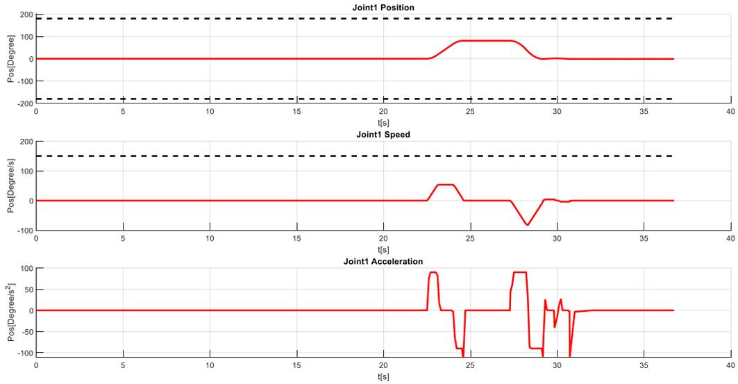
Figure 0-8 IRB 1600: Joint 1 – position, speed and acceleration profiles
