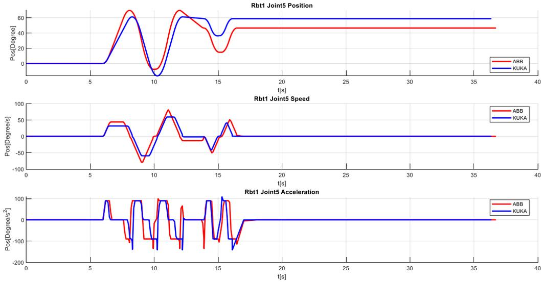
Figure 0-30 IRB1200 vs KR6 r700: Joint 5 – position, speed and acceleration profiles
