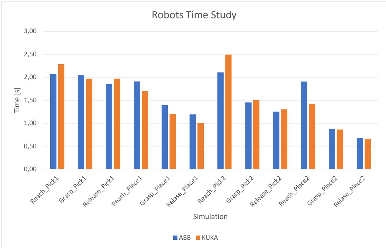
Figure 0-40 Robots time study – setups comparison
