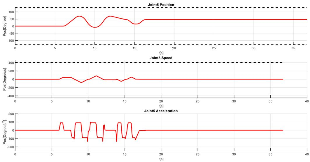
Figure 0-6 IRB 1200: Joint 5 – position, speed and acceleration profiles
