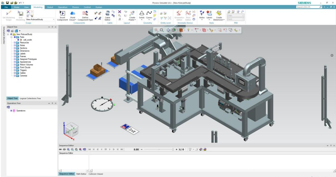
Figure 0-14 Present Conveyor System Process Simulate model once imported
