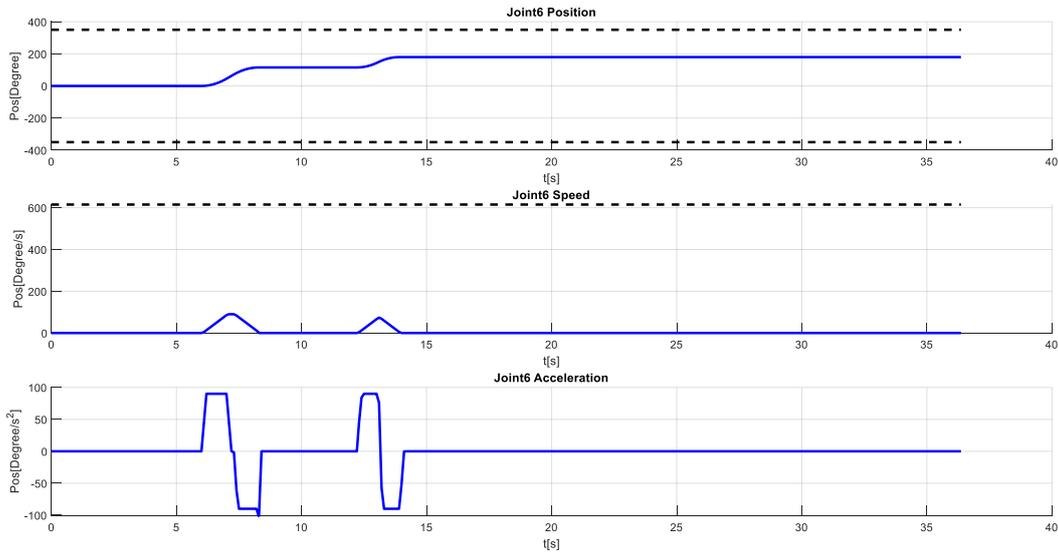
Figure 0-19 KR6 r700: Joint 6 – position, speed and acceleration profiles
