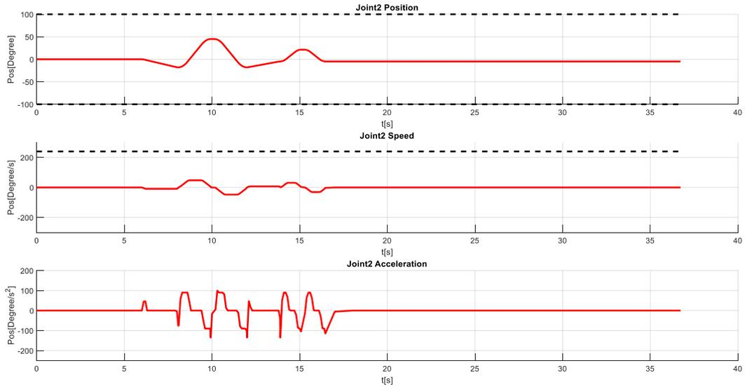
Figure 0-3 IRB 1200: Joint 2 – position, speed and acceleration profiles
