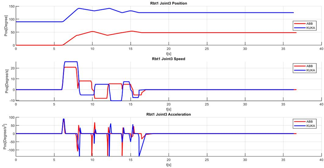
Figure 0-28 IRB1200 vs KR6 r700: Joint 3 – position, speed and acceleration profiles
