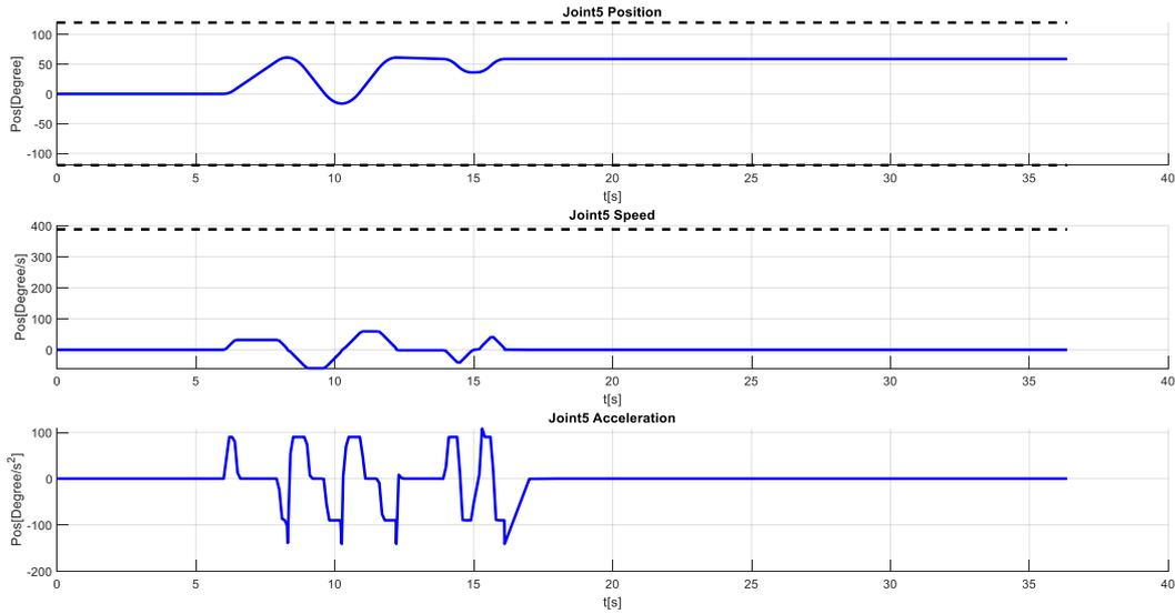
Figure 0-18 KR6 r700: Joint 5 – position, speed and acceleration profiles
