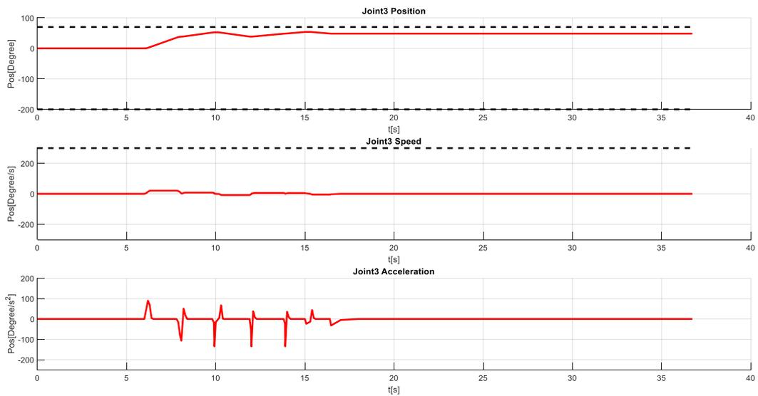
Figure 0-4 IRB 1200: Joint 3 – position, speed and acceleration profiles
