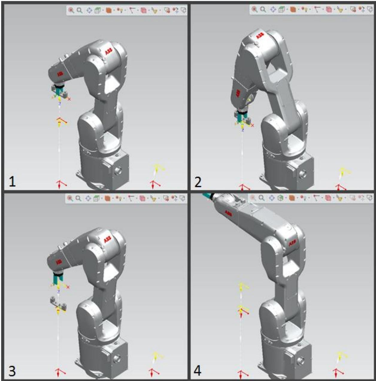
Figure 0-6 IRB 1600 place poses: 1 via (approach) location, 2 place location, 3 via (retract) location, 4 home
