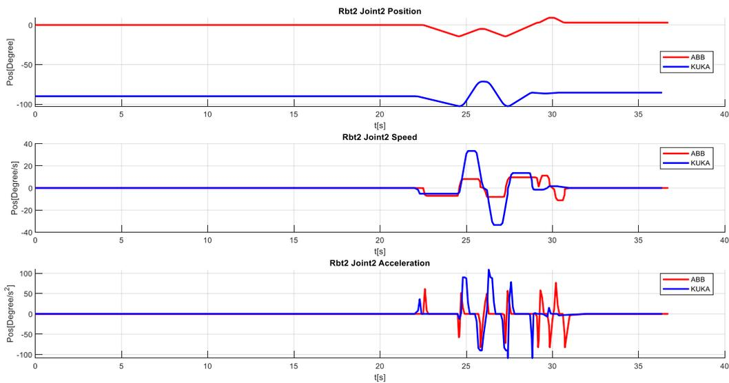
Figure 0-33 IRB1600 vs KR10 r1100: Joint 2 – position, speed and acceleration profiles
