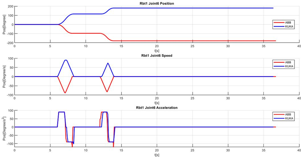
Figure 0-31 IRB1200 vs KR6 r700: Joint 6 – position, speed and acceleration profiles
