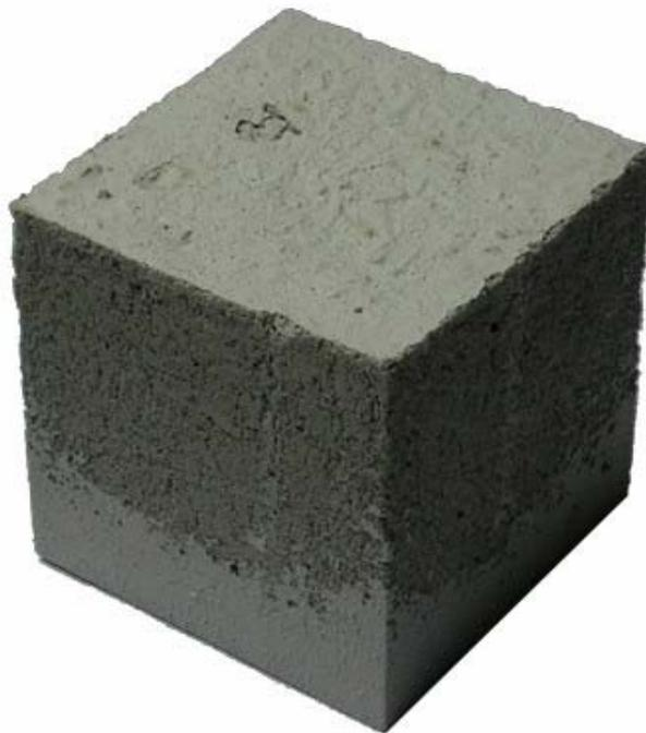
Provino cubico in Mineralized Wood Concrete
