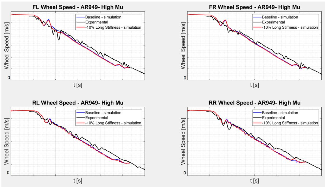
Figure 10.14.1 – Estimated wheel speed – Baseline vs -10% Structural longitudinal stiffness
