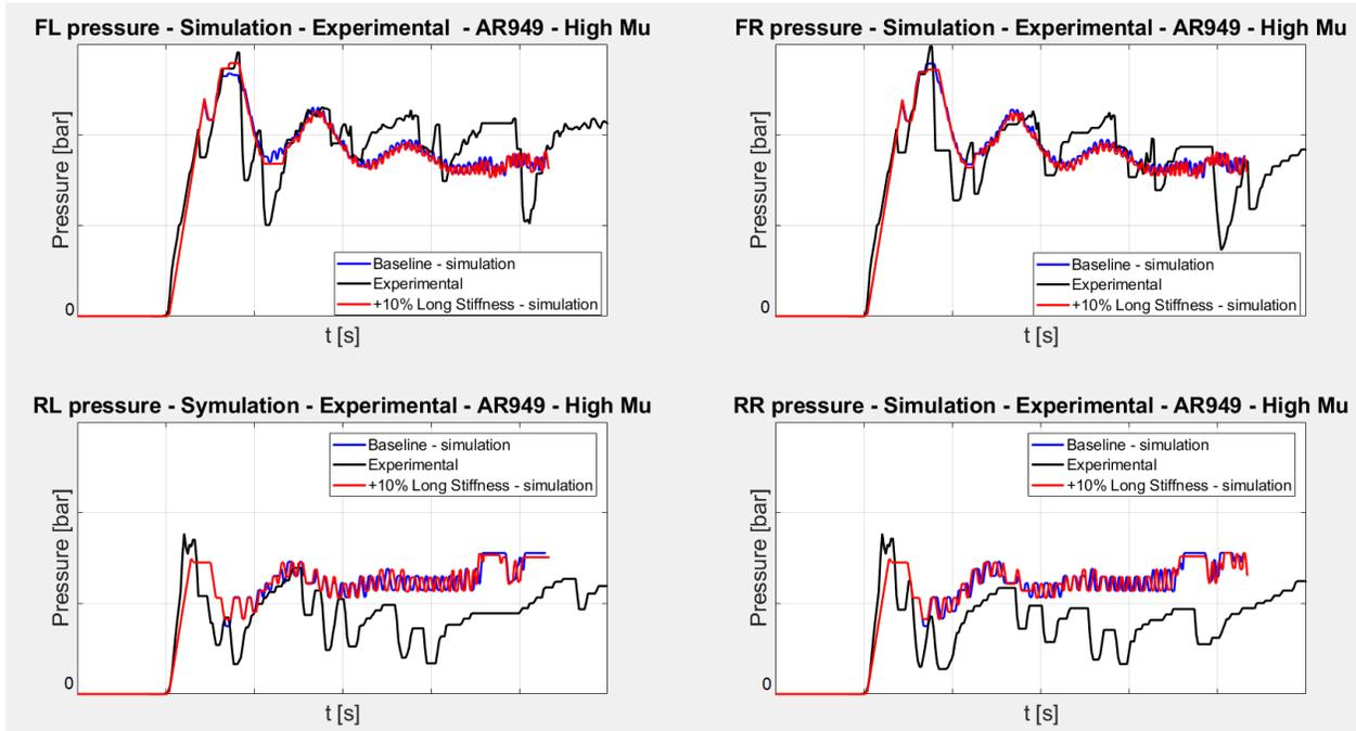
Figure 10.13.2 – Brake pressure on the four corners – Baseline vs +10% Structural longitudinal stiffness
