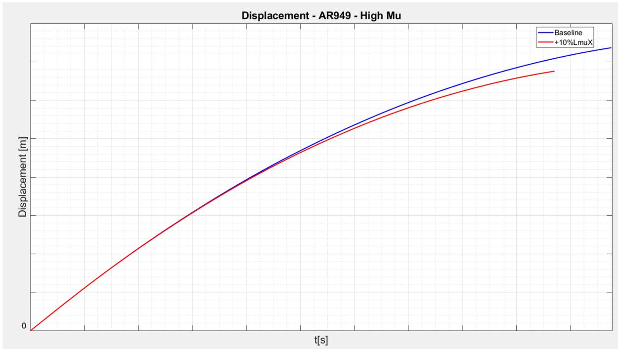
Figure 10.3.4 – Braking distance – Baseline vs +10%LMUX
