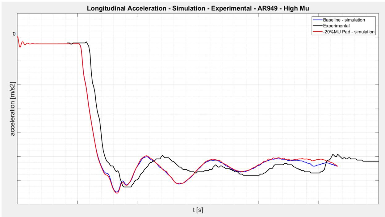
Figure 10.10.4 – Vehicle longitudinal acceleration – Baseline vs -20% Pad's Mu
