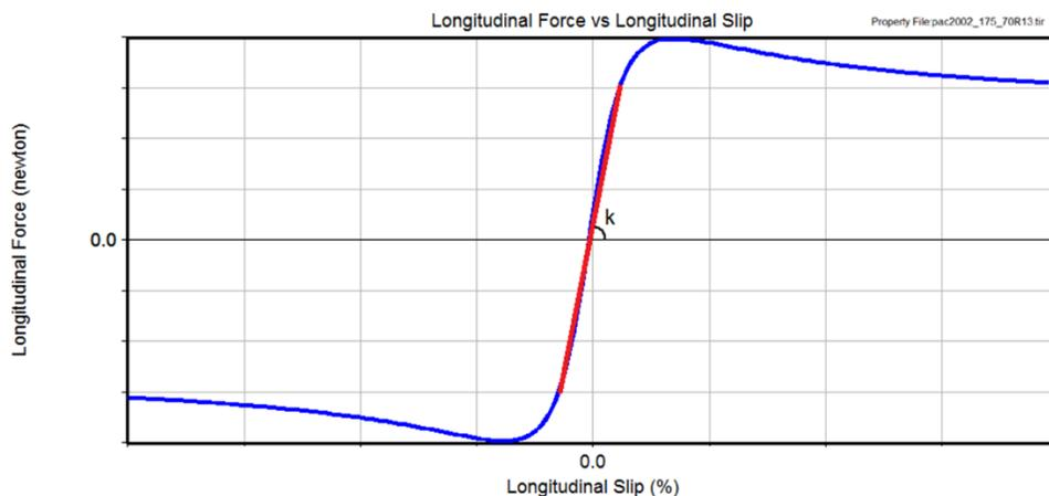
Figure 8.19 - Longitudinal force versus longitudinal slip, with the slope K for small slip values
