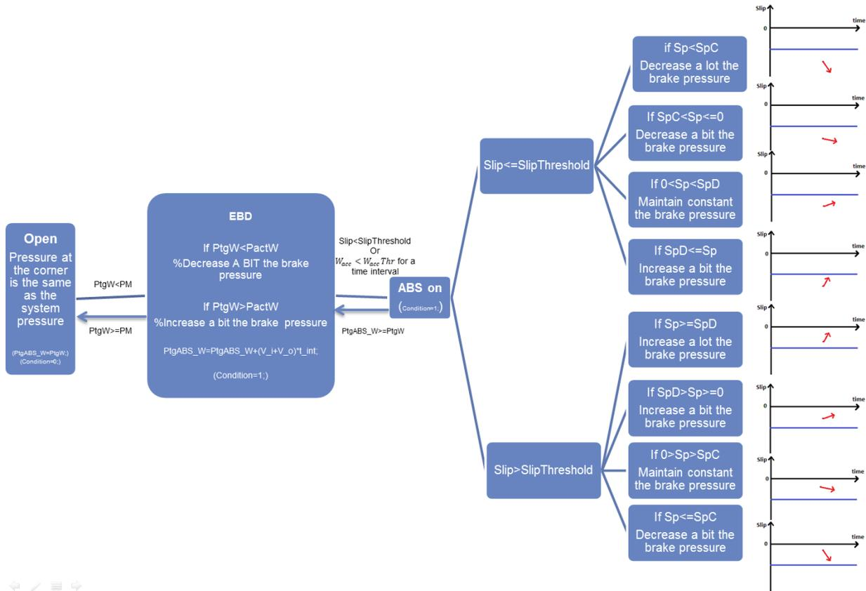
Figure 8.23 - Schematic representation of ABS rear valves logic
