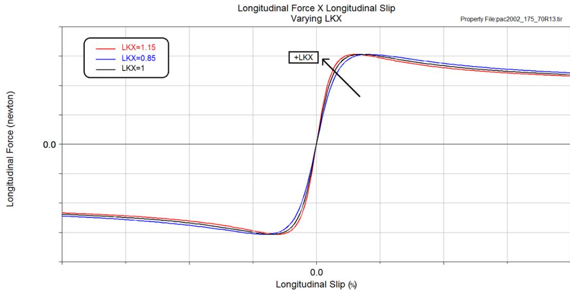
Figure 10.5 - Curves  $F_x(\sigma)$  for 175/70 R 15 tire obtained for different values of LKX.
