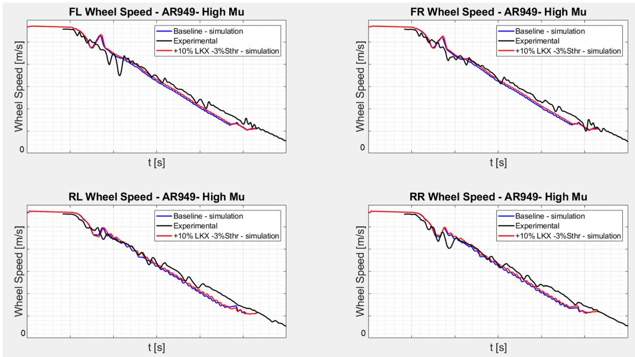
Figure 10.8.1 – Estimated wheel speed – Baseline vs +10%LKX -3%Sthr
