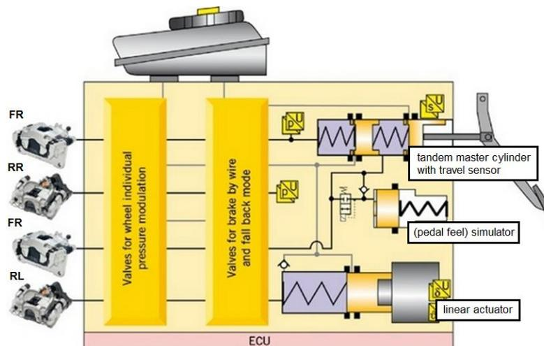
Figure 6.3 – Integrated Brake System (IBS) model [3]
