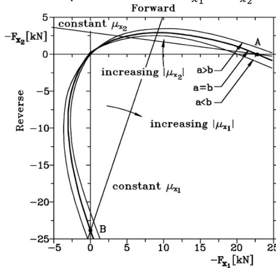
Figure 4.2 – Braking in ideal conditions. Relationship between  $F_{x_1}$  and  $F_{x_2}$
