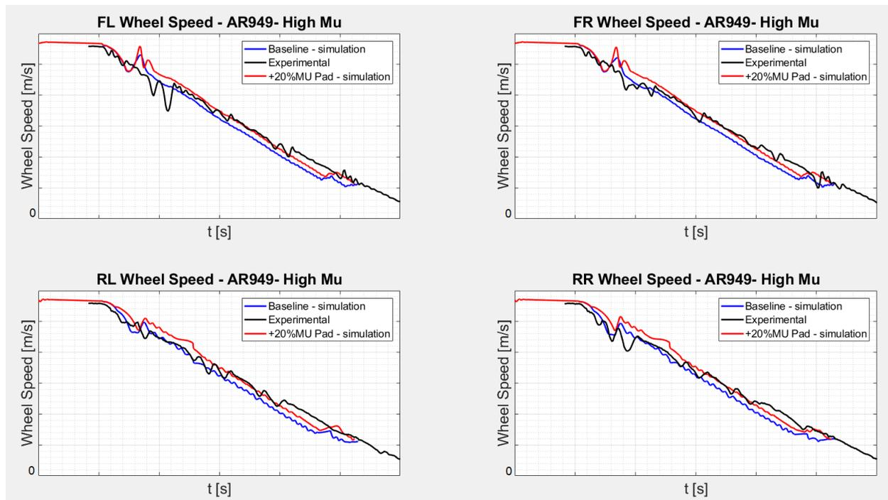
Figure 10.9.1 – Estimated wheel speed – Baseline vs +20% Pad's  $\mu$
