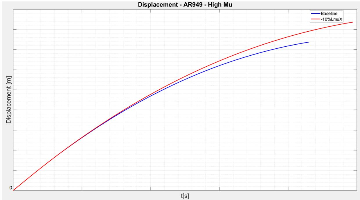
Figure 10.4.4 – Braking distance – Baseline vs -10%LMUX
