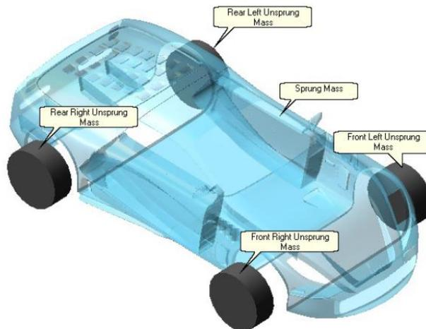
Figure 2.2 - CarRealTime vehicle simplified model
