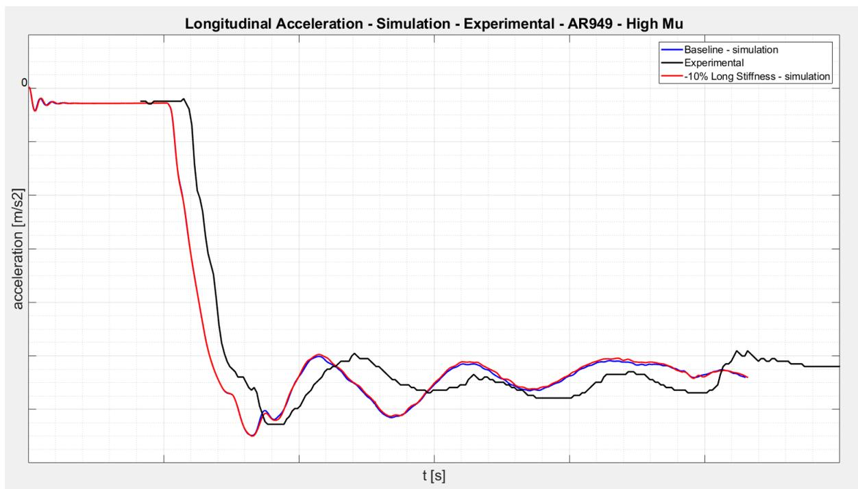
Figure 10.14.3 – Vehicle longitudinal acceleration – Baseline vs -10% Structural longitudinal stiffness
