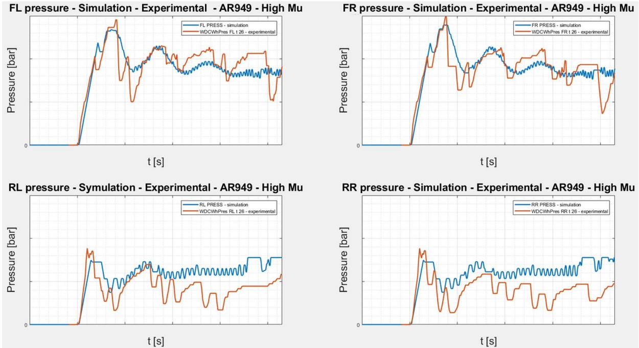
Figure 9.1.4 – Brake pressure on the four corners – AR949 on dry road
