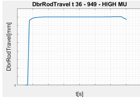
Figure 8.2 - Brake pedal pushrod travel – Experimental data
