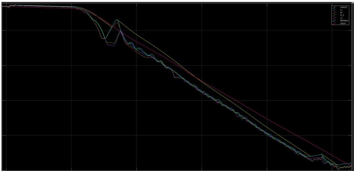
Figure 9.1.3 – Estimated vehicle speed (yellow) and estimated wheel speeds – AR949 on dry road
