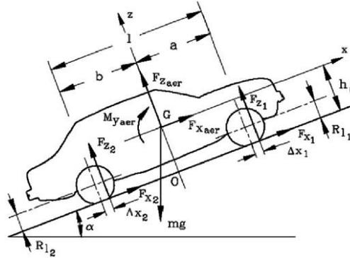
Figure 4.1 - Forces acting on a vehicle moving on an inclined road
