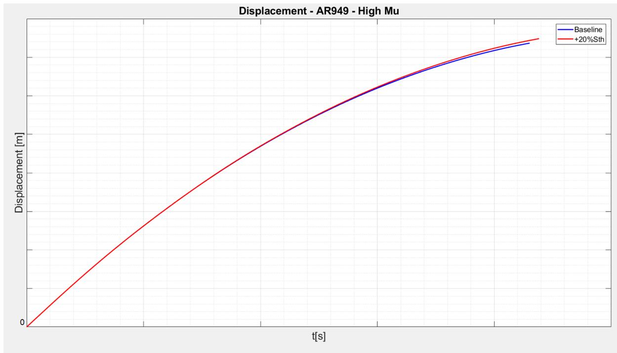
Figure 10.11.4 – Braking distance – Baseline vs +20%Sthr
