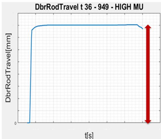
Figure 8.6 - Brake pedal pushrod travel- Experimental data
