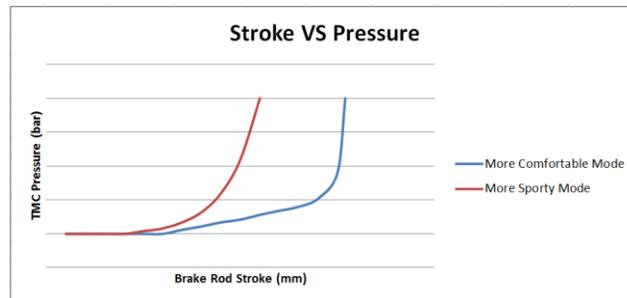
Figure 6.2 – Continental's Pushrod travel vs Pushrod force and Pressure. Comfort and Sport mode
