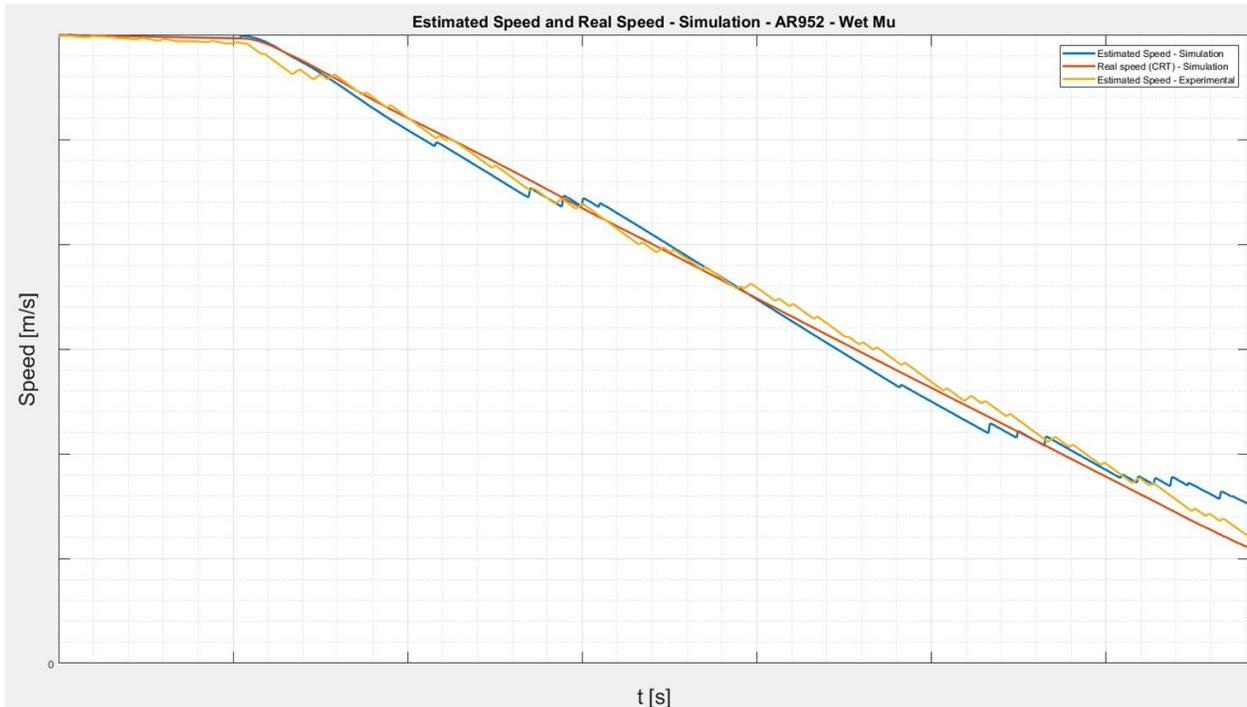
Figure 9.2.2 – Estimated vehicle speed – AR952 on wet road
