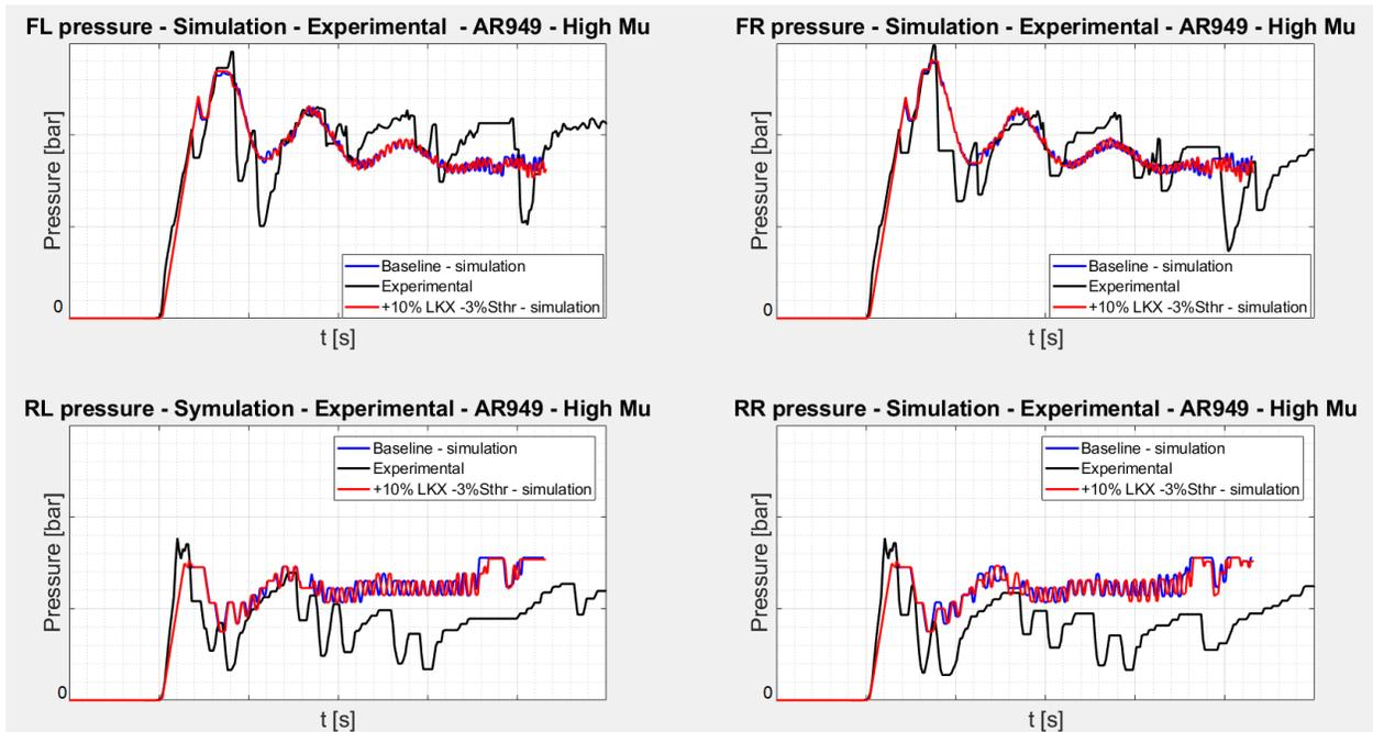
Figure 10.8.2 – Brake pressure on the four corners – Baseline vs +10%LKX -3%Sthr
