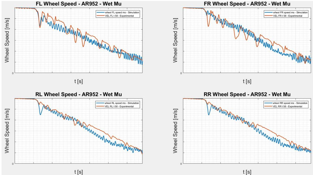
Figure 9.2.1 – Estimated wheel speed – AR952 on wet road
