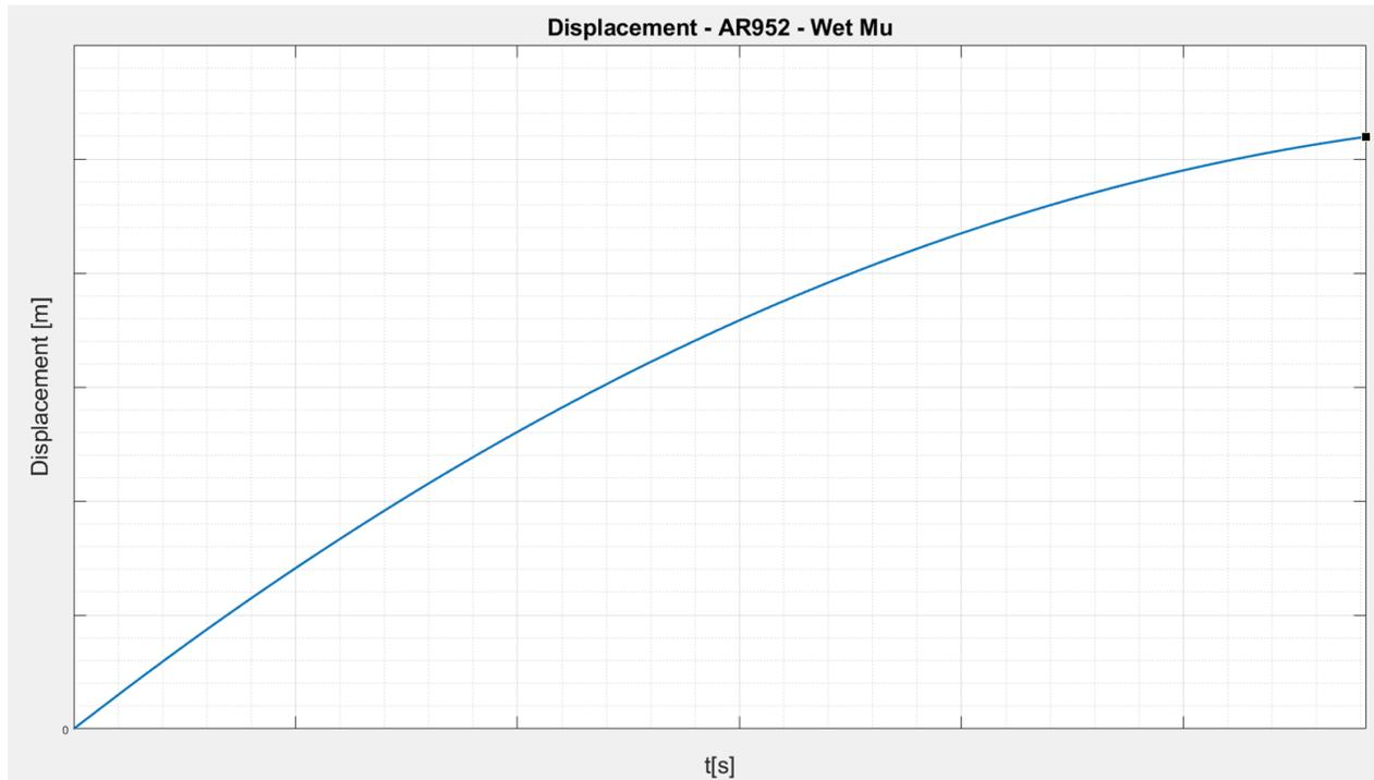
Figure 9.2.7 – Braking distance – AR952 on wet road
