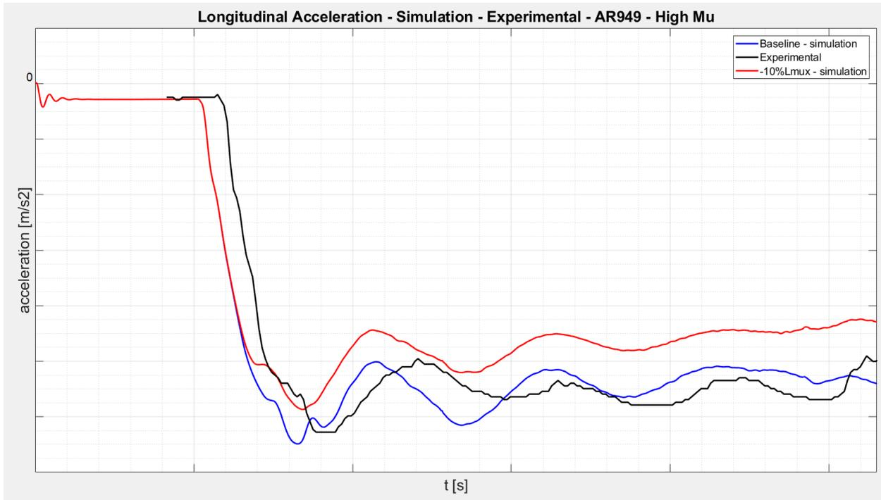
Figure 10.4.3 – Vehicle longitudinal acceleration – Baseline vs -10%LMUX
