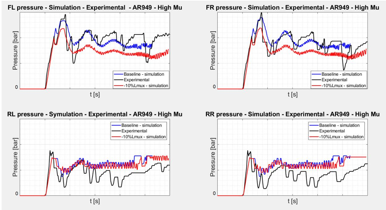
Figure 10.4.2 – Brake pressure on the four corners – Baseline vs -10%LMUX
