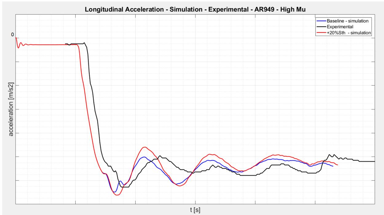
Figure 10.11.3 – Vehicle longitudinal acceleration – Baseline vs +20%Sthr
