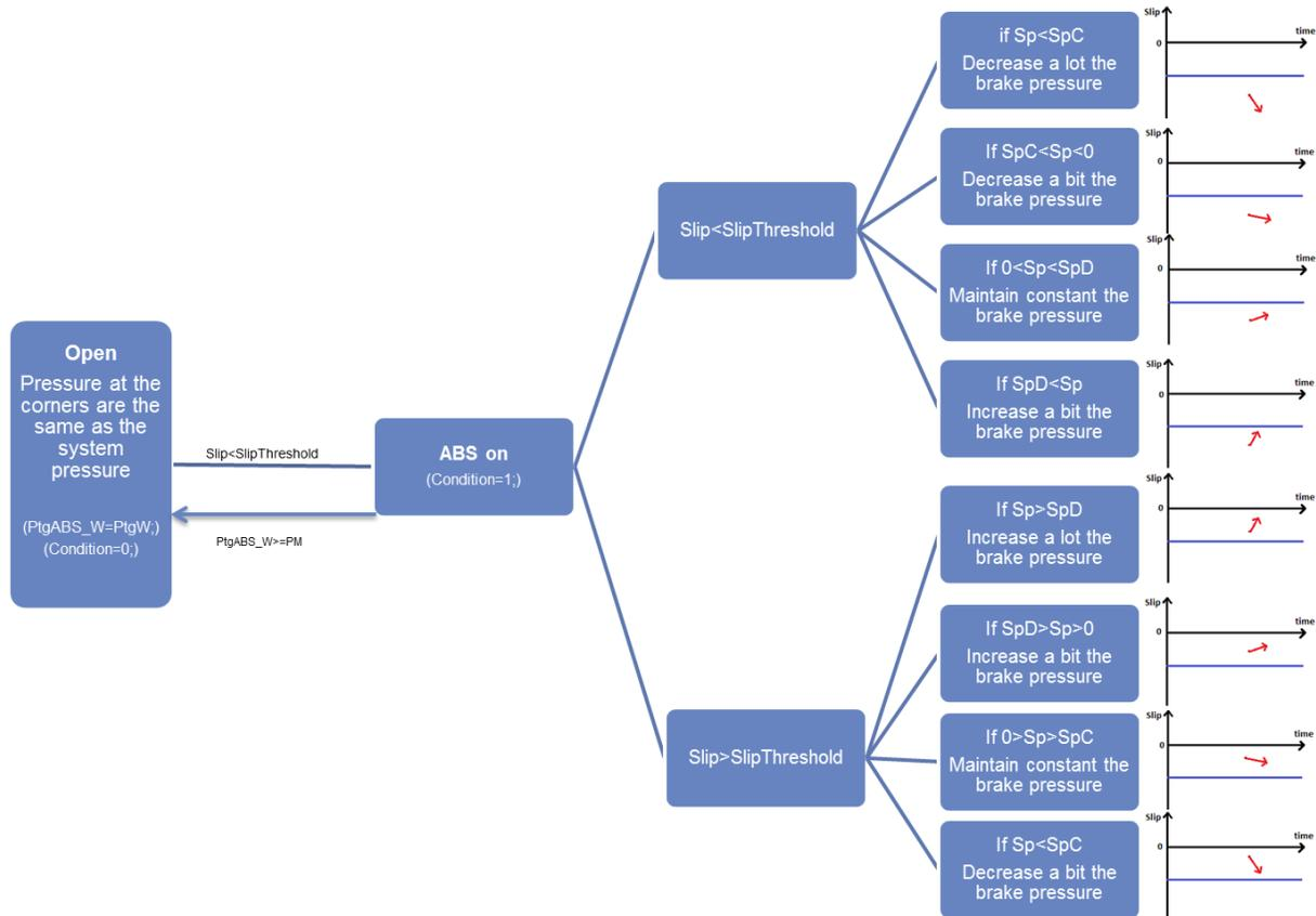
Figure 8.22 - Schematic representation of ABS front valves logic
