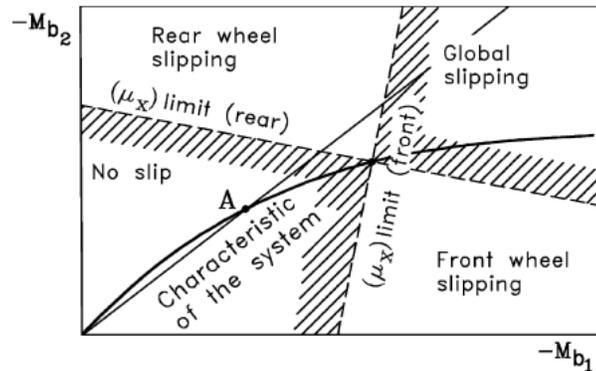
Figure 4.4 - Conditions for ideal braking, characteristic line for a system with constant  $K_b$
