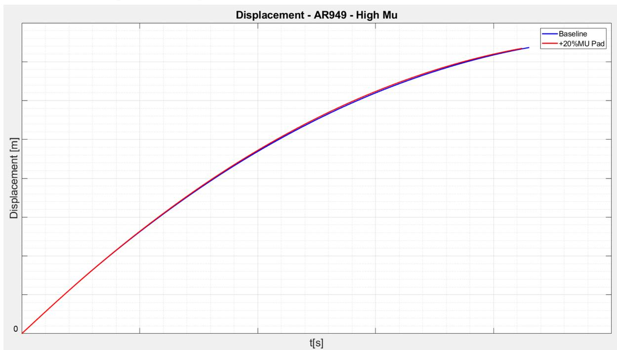
Figure 10.9.5 – Braking distance – Baseline vs +20% Pad's Mu
