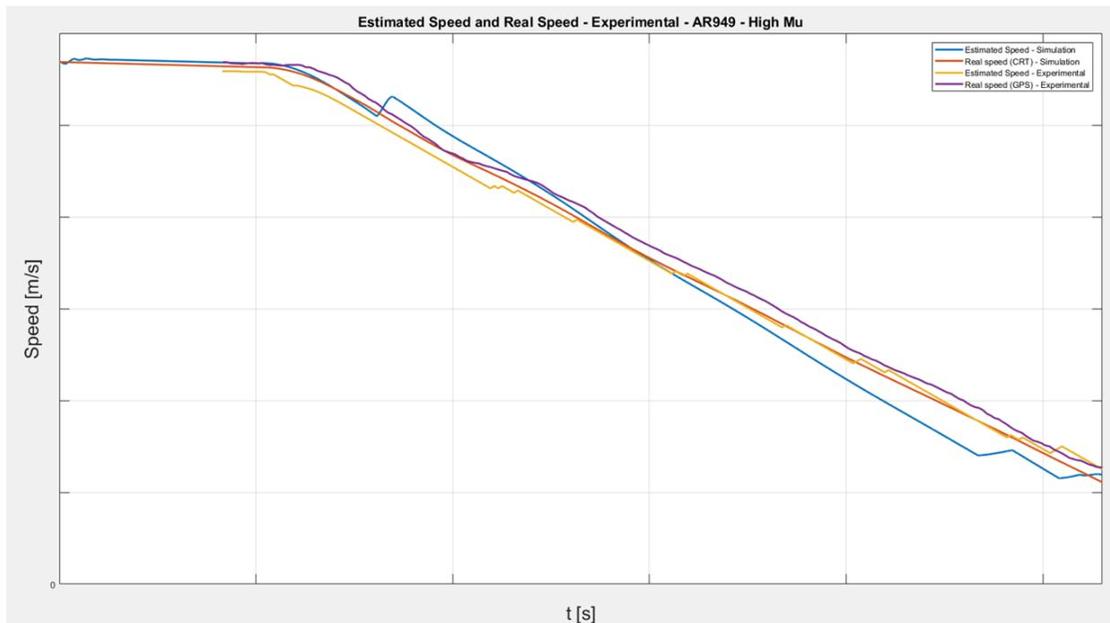
Figure 9.1.2 – Estimated vehicle speed – AR949 on dry road
