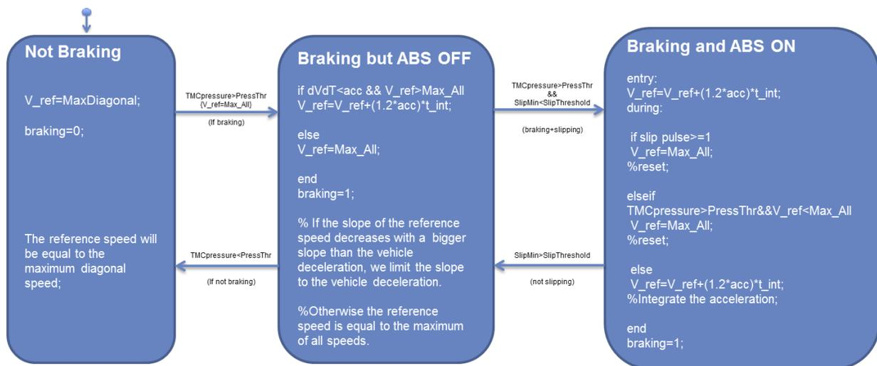
Figure 8.14 - Speed estimator logic
