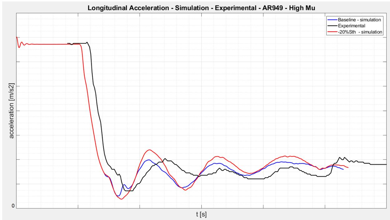
Figure 10.12.3 – Vehicle longitudinal acceleration – Baseline vs -20%Sthr
