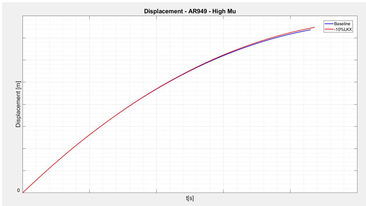
Figure 10.7.4 – Braking distance – Baseline vs -10%LXX
