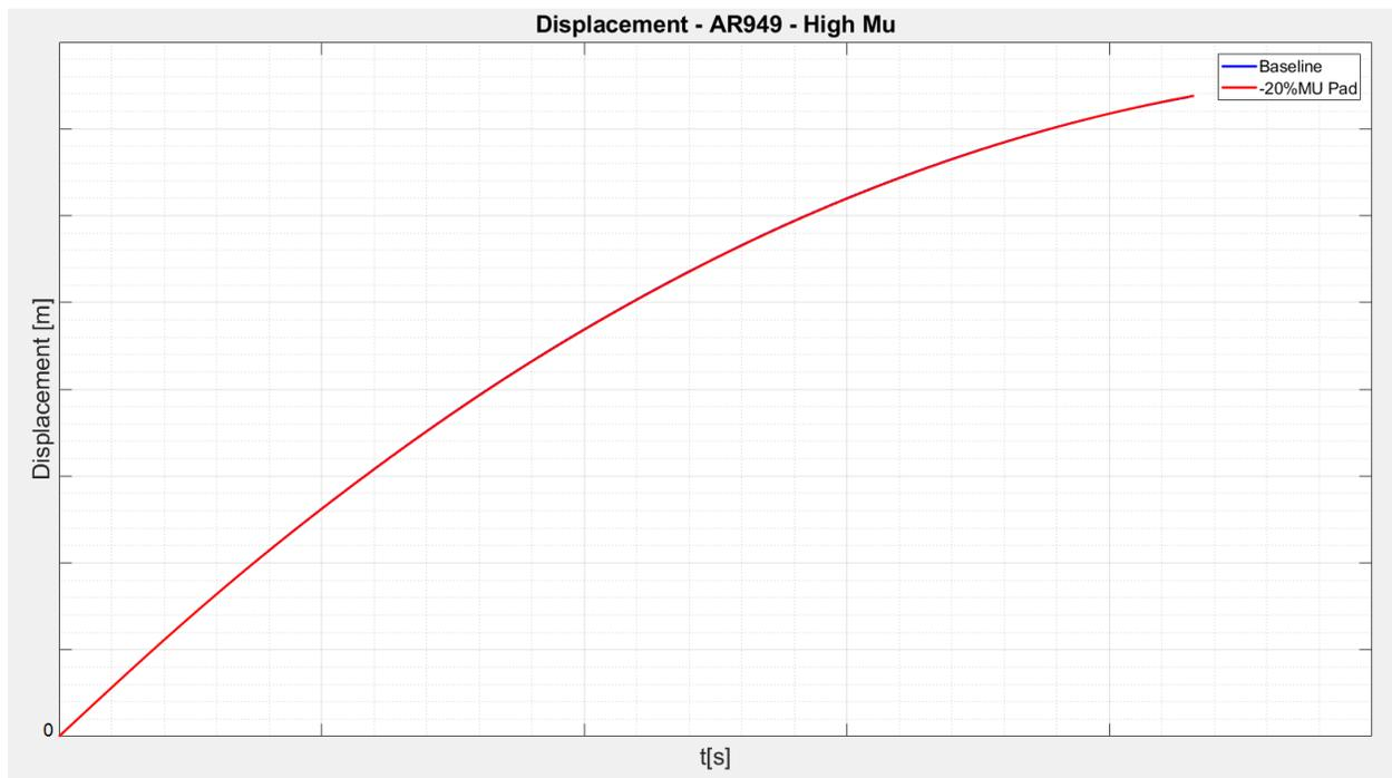
Figure 10.10.5 – Braking distance – Baseline vs -20% Pad's Mu
