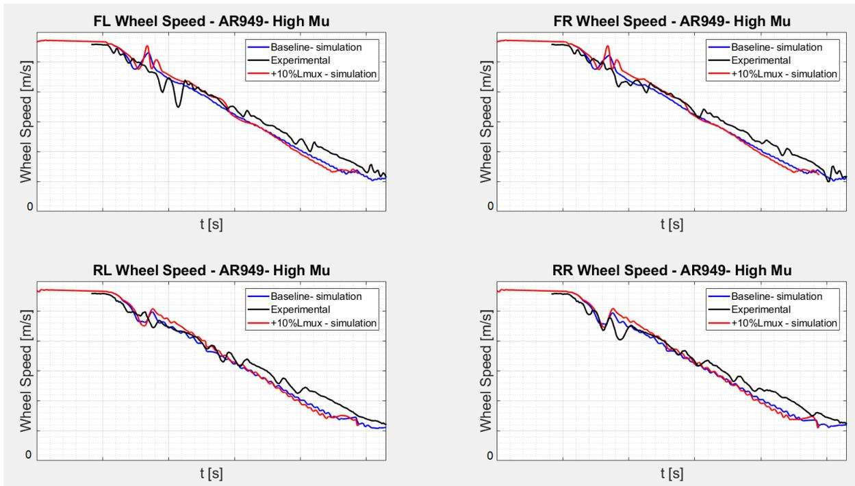
Figure 10.3.1 – Estimated wheel speed – Baseline vs +10%LMUX
