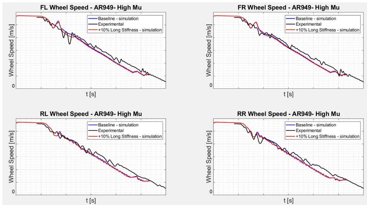
Figure 10.13.1 – Estimated wheel speed – Baseline vs +10% Structural longitudinal stiffness
