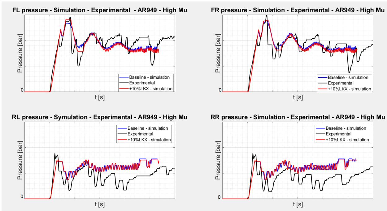
Figure 10.6.2 – Brake pressure on the four corners – Baseline vs +10%LKK
