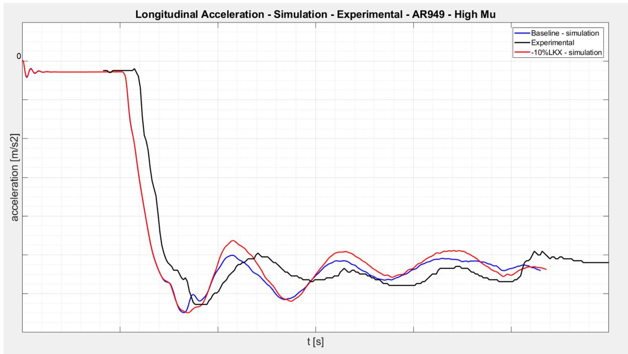
Figure 10.7.3 – Vehicle longitudinal acceleration – Baseline vs -10%LKX
