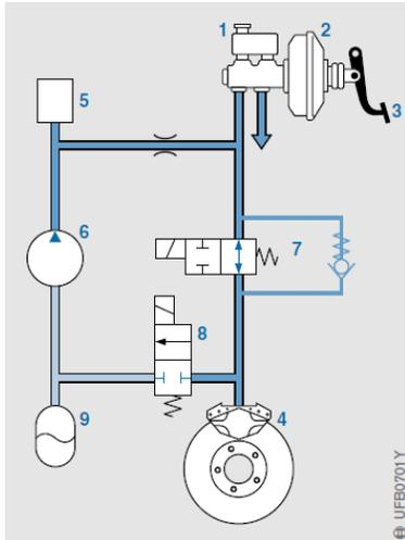
Figure 5.2 - Principle of hydraulic modulator with 2/2 solenoid valves (schematic)
