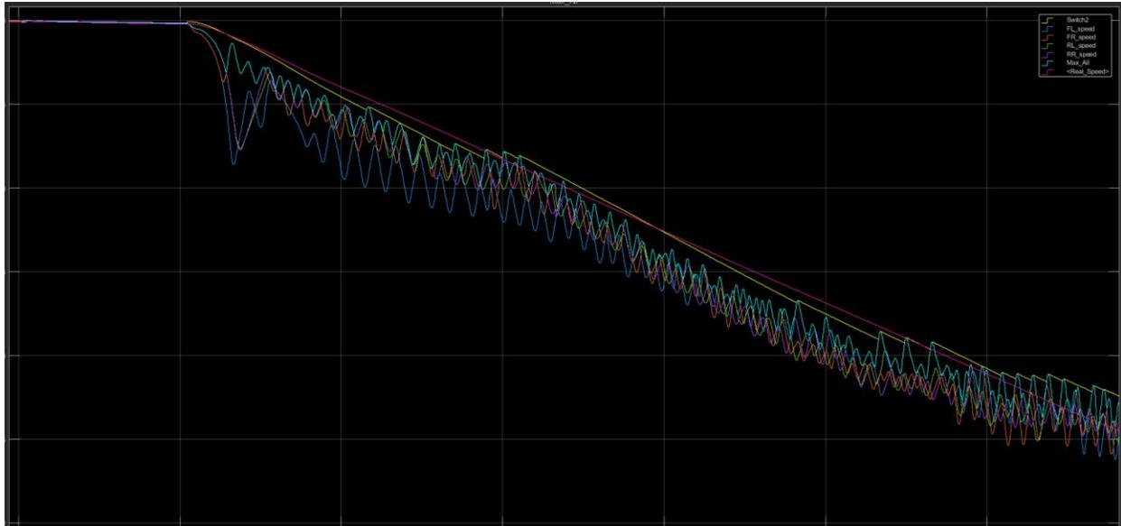
Figure 9.2.3 – Estimated vehicle speed (yellow) and estimated wheel speeds – AR952 on wet road
