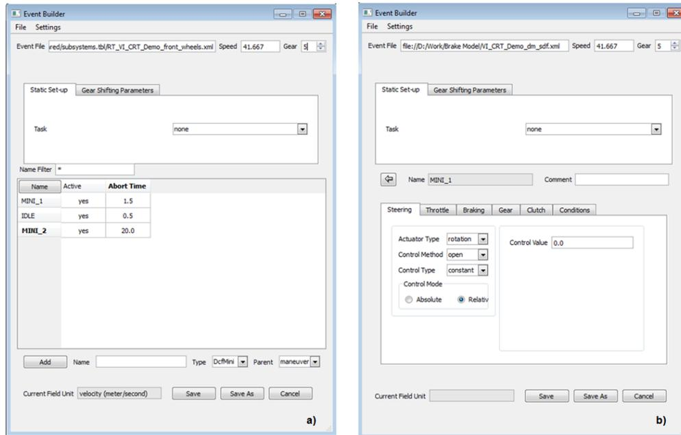
Figure 2.10- (a) Driving Machine file; (b) Mini maneuver
