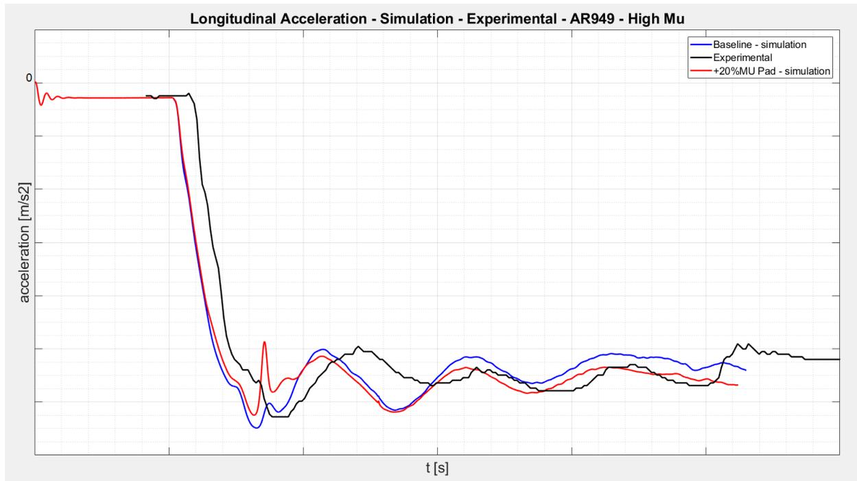
Figure 10.9.4 – Vehicle longitudinal acceleration – Baseline vs +20% Pad's Mu
