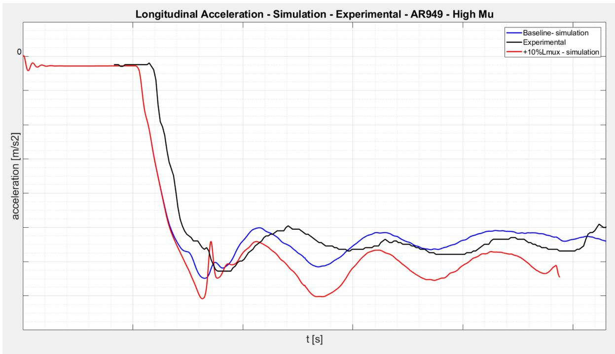
Figure 10.3.3 – Vehicle longitudinal acceleration – Baseline vs +10%LMUX
