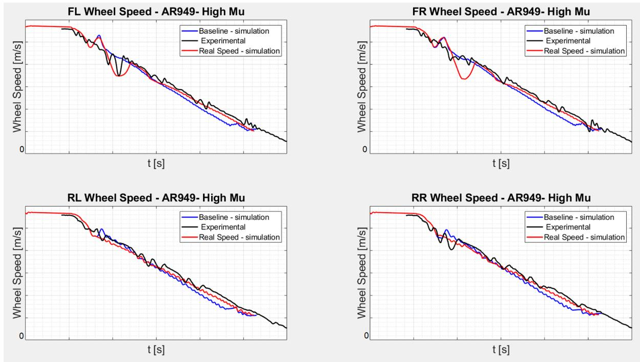
Figure 10.1.1 – Estimated wheel speed – Baseline vs CRT real speed
