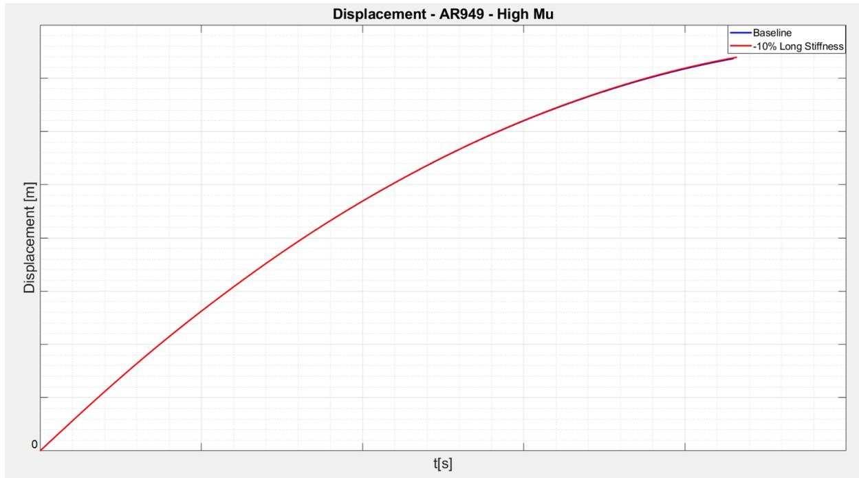
Figure 10.14.4 – Braking distance – Baseline vs -10% Structural longitudinal stiffness
