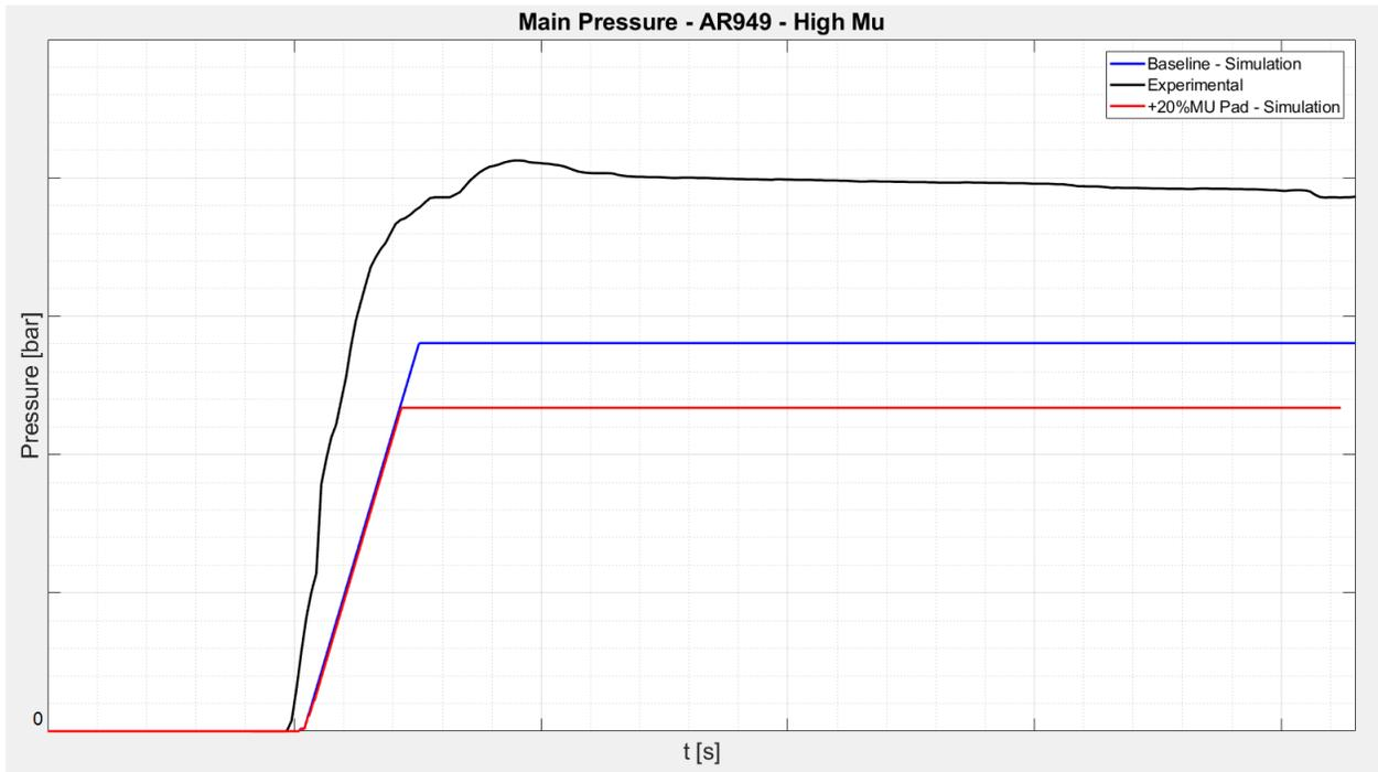
Figure 10.9.3 – Main System Pressure – Baseline vs +20% Pad’s Mu
