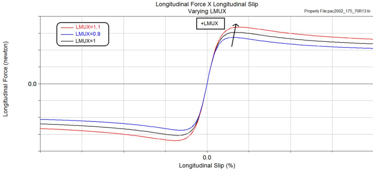
Figure 10.2 - Curves  $F_x(\sigma)$  for 175/70 R 15 tire obtained for different values of LMUX.
