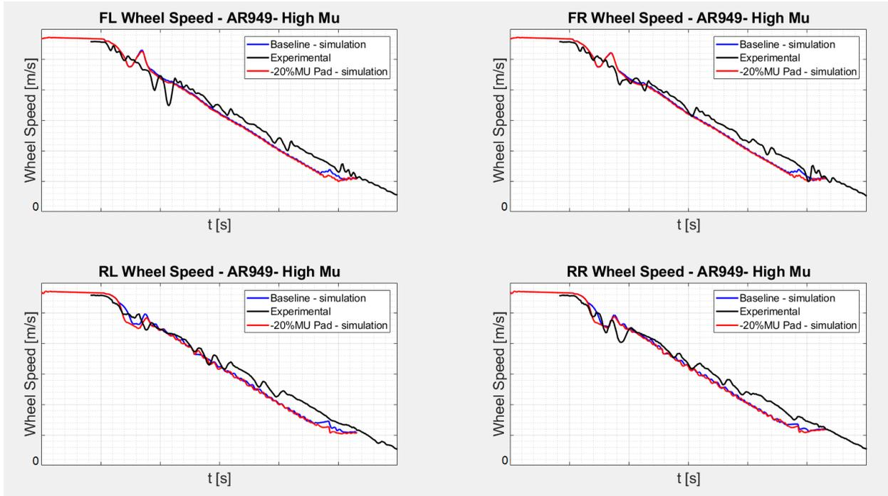
Figure 10.10.1 – Estimated wheel speed – Baseline vs -20% Pad's Mu
