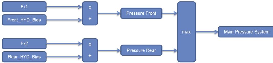
Figure 8.12 - Schematic representation of obtaining the main pressure of the system
