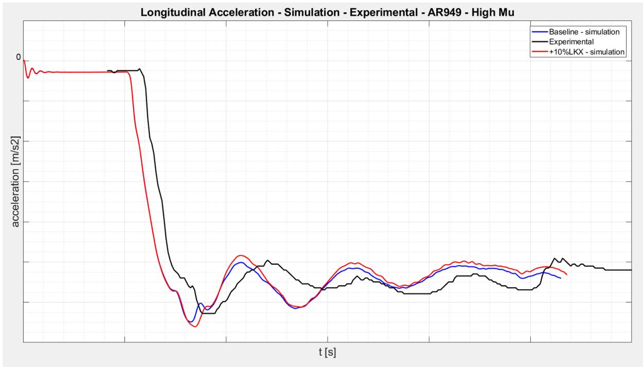
Figure 10.6.3 – Vehicle longitudinal acceleration – Baseline vs +10%LKK
