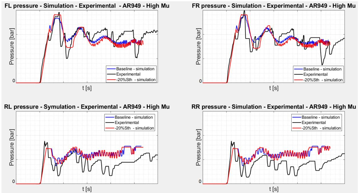
Figure 10.12.2 – Brake pressure on the four corners – Baseline vs -20%Sthr
