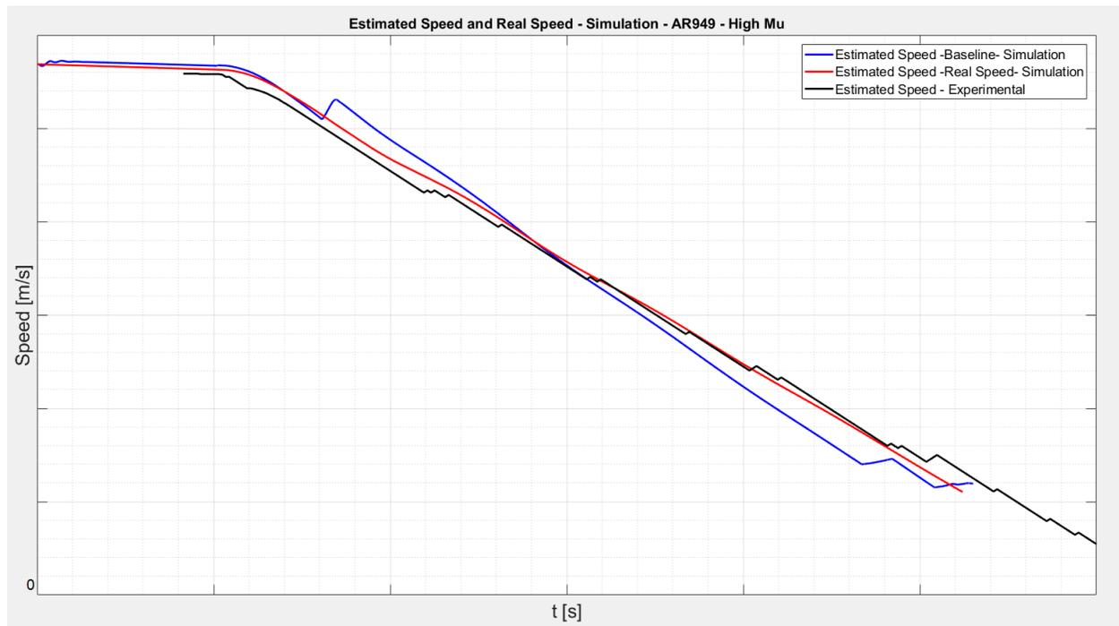
Figure 10.1.2 – Estimated vehicle speed – Baseline vs CRT real speed
