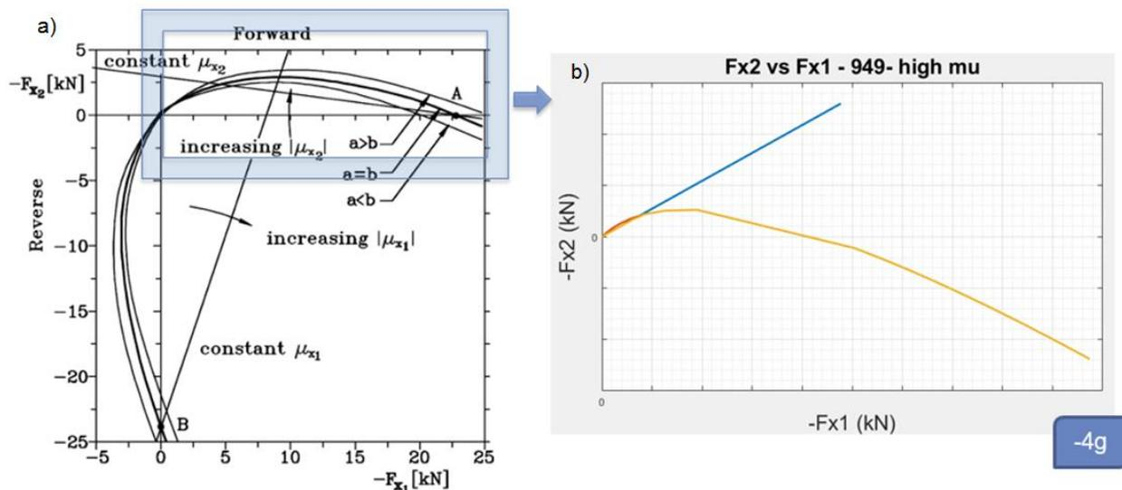
Figure 8.11- Braking in ideal conditions. Relationship between  $F_{x_1}$  and  $F_{x_2}$ . (a) Theoretical; (b) Simulation
