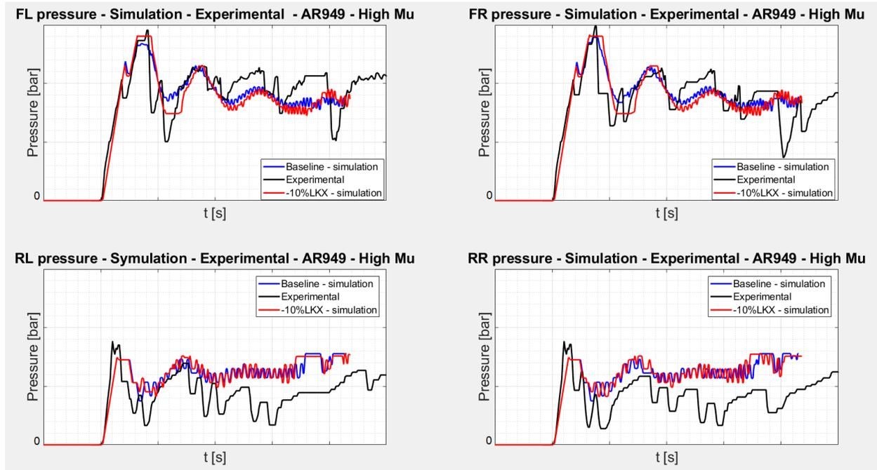
Figure 10.7.2 – Brake pressure on the four corners – Baseline vs -10%LKX
