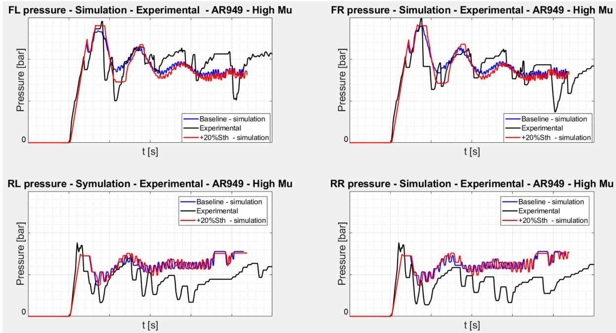
Figure 10.11.2 – Brake pressure on the four corners – Baseline vs +20%Sth
