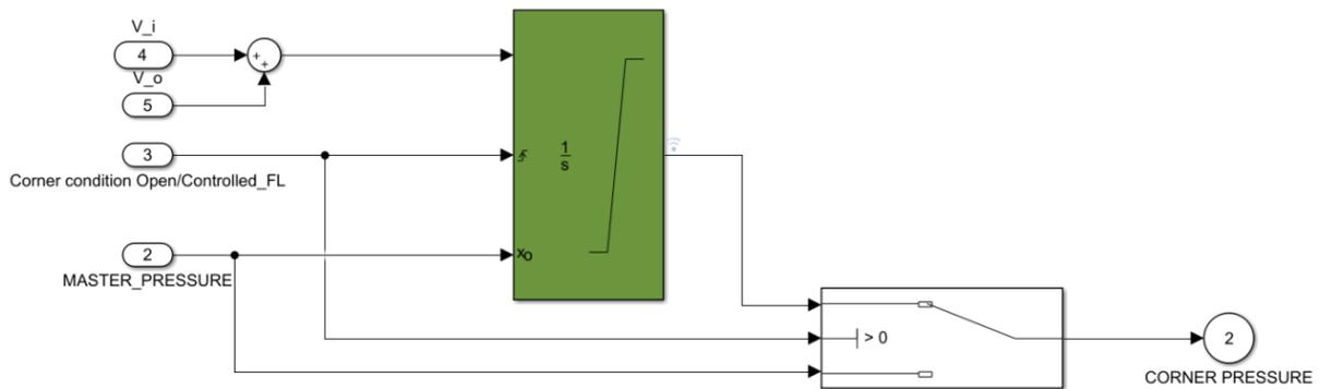
Figure 8.25 –Valve physical model blocks
