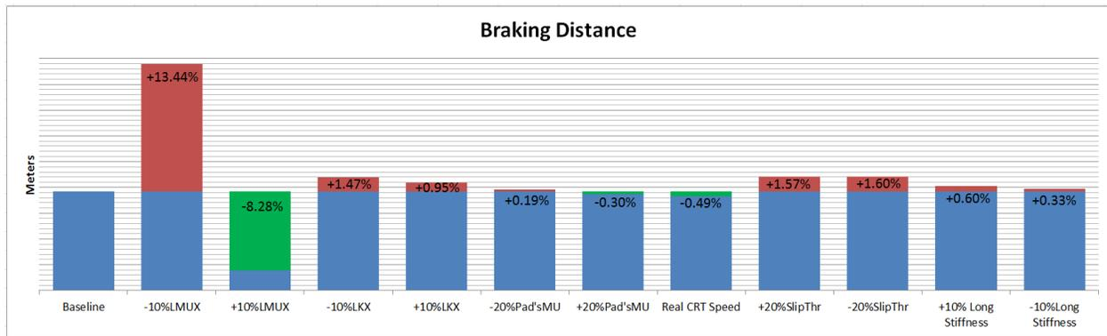
Figure 10.15 – Histogram Braking distance – Sensitivity Analysis - Overall results
