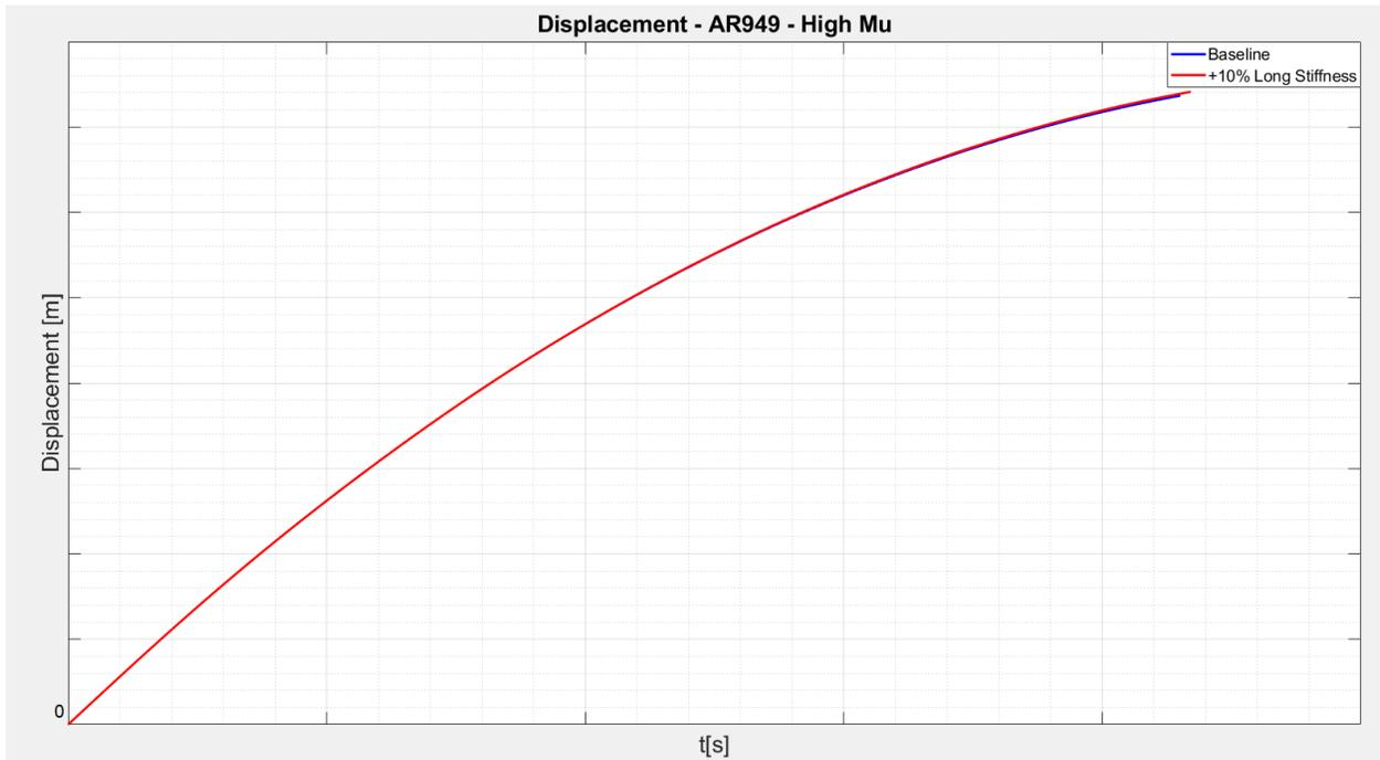
Figure 10.13.4 – Braking distance – Baseline vs +10% Structural longitudinal stiffness
