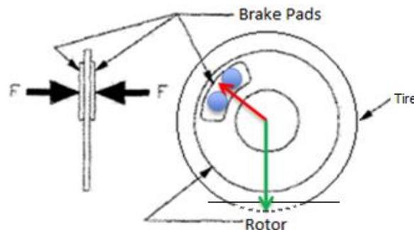
Figure 8.13 – Disk brake configuration example
