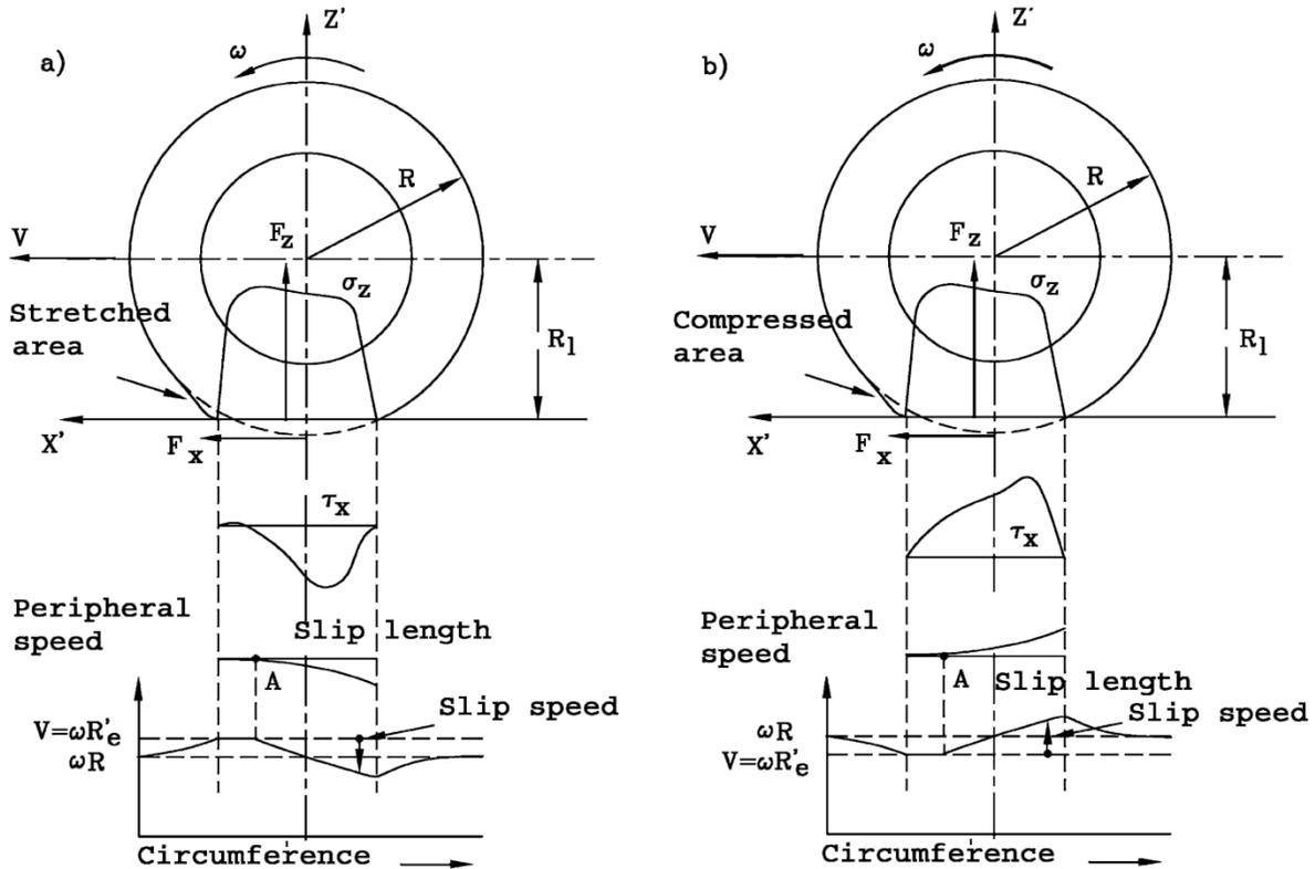
Figure 3.2 –Contact pressure distribution for braking (a) and driving (b) wheel.
