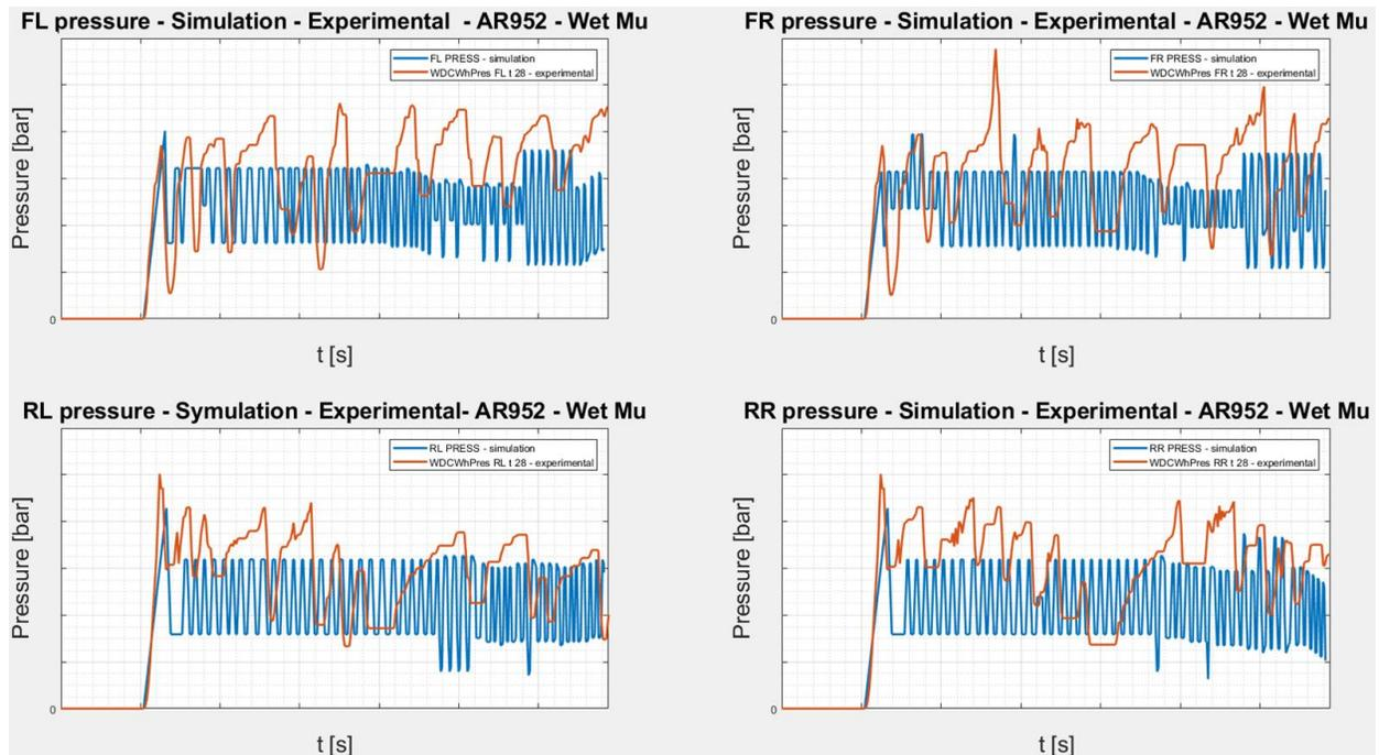
Figure 9.2.4 – Brake pressure on the four corners – AR952 on wet road
