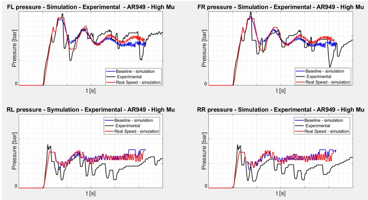
Figure 10.1.3 – Brake pressure on the four corners – Baseline vs CRT real speed
