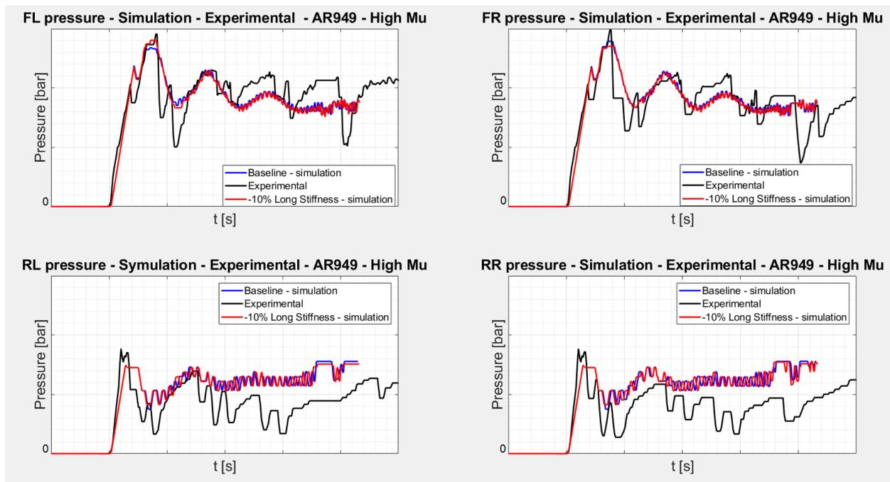
Figure 10.14.2 – Brake pressure on the four corners – Baseline vs -10% Structural longitudinal stiffness
