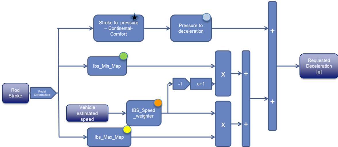
Figure 8.3 - Schematic representation of obtaining driver's desired deceleration
