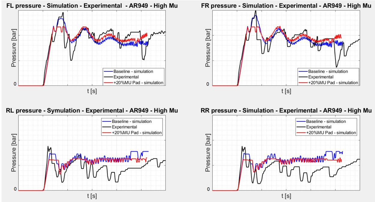
Figure 10.9.2 – Brake pressure on the four corners – Baseline vs +20% Pad’s Mu
