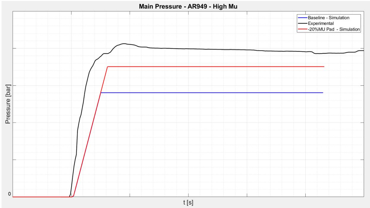
Figure 10.10.3 – Main System Pressure – Baseline vs -20% Pad's Mu
