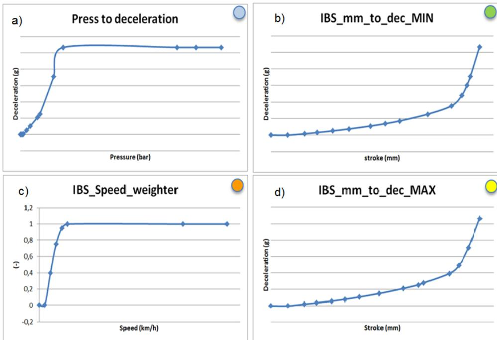
Figure 8.4 - Plots of the blocks used in the scheme for obtain the driver's desired deceleration
