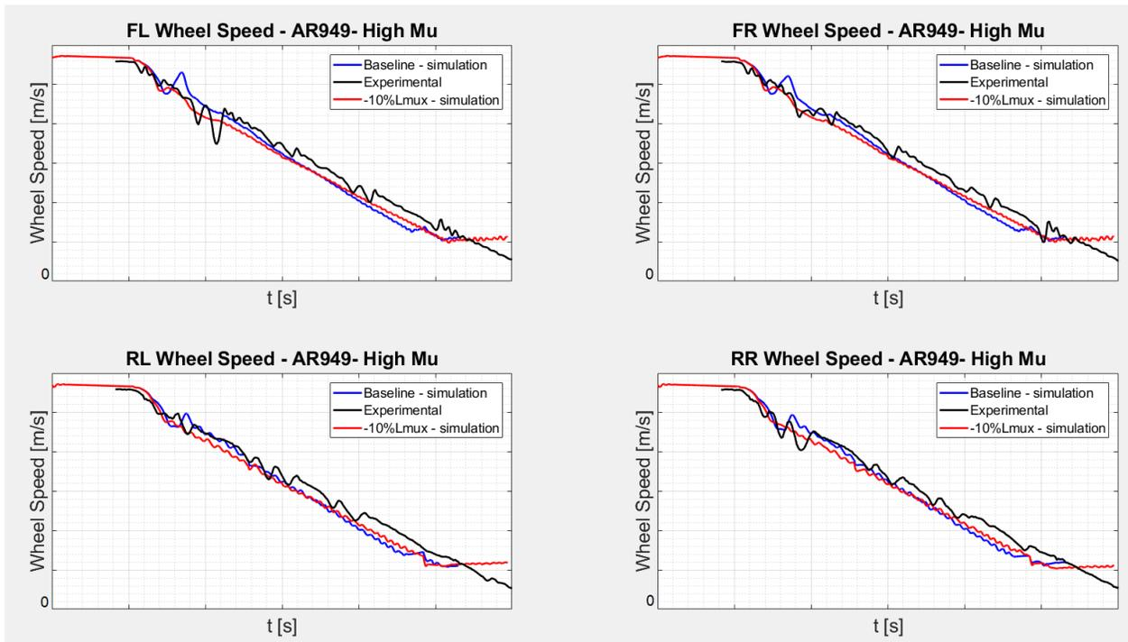
Figure 10.4.1 – Estimated wheel speed – Baseline vs -10%LMUX
