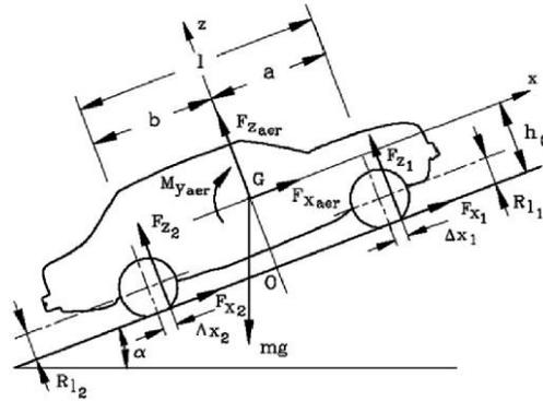
Figure 8.10 - Forces acting on a vehicle moving on an inclined road
