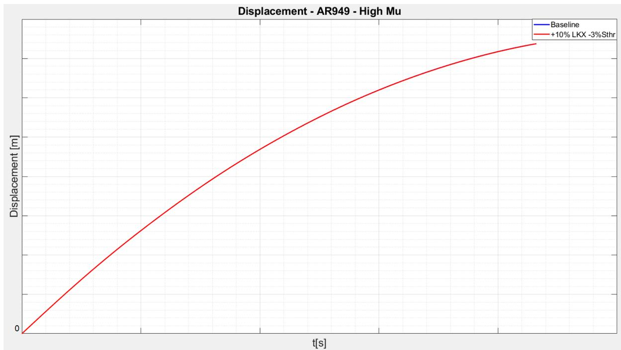
Figure 10.8.4 – Braking distance – Baseline vs +10%LKX -3%Sthr
