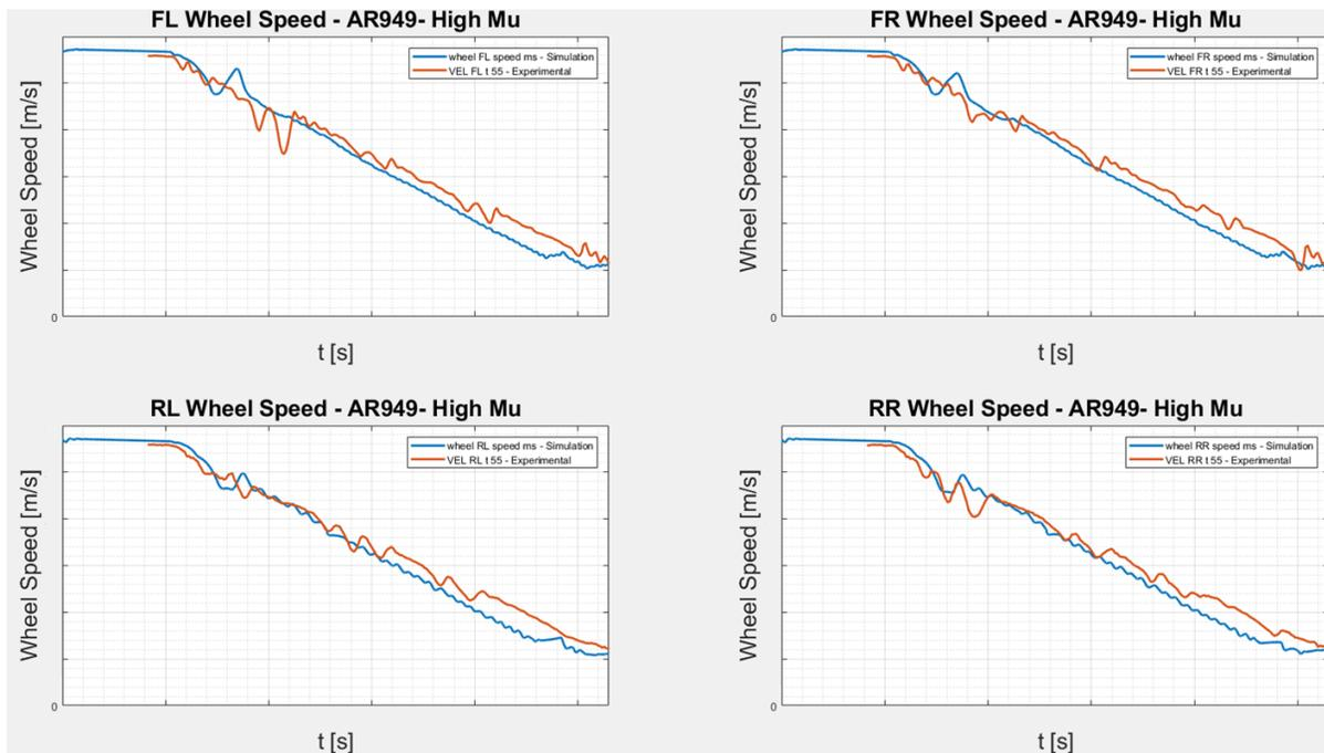
Figure 9.1.1 – Estimated wheel speed – AR949 on dry road
