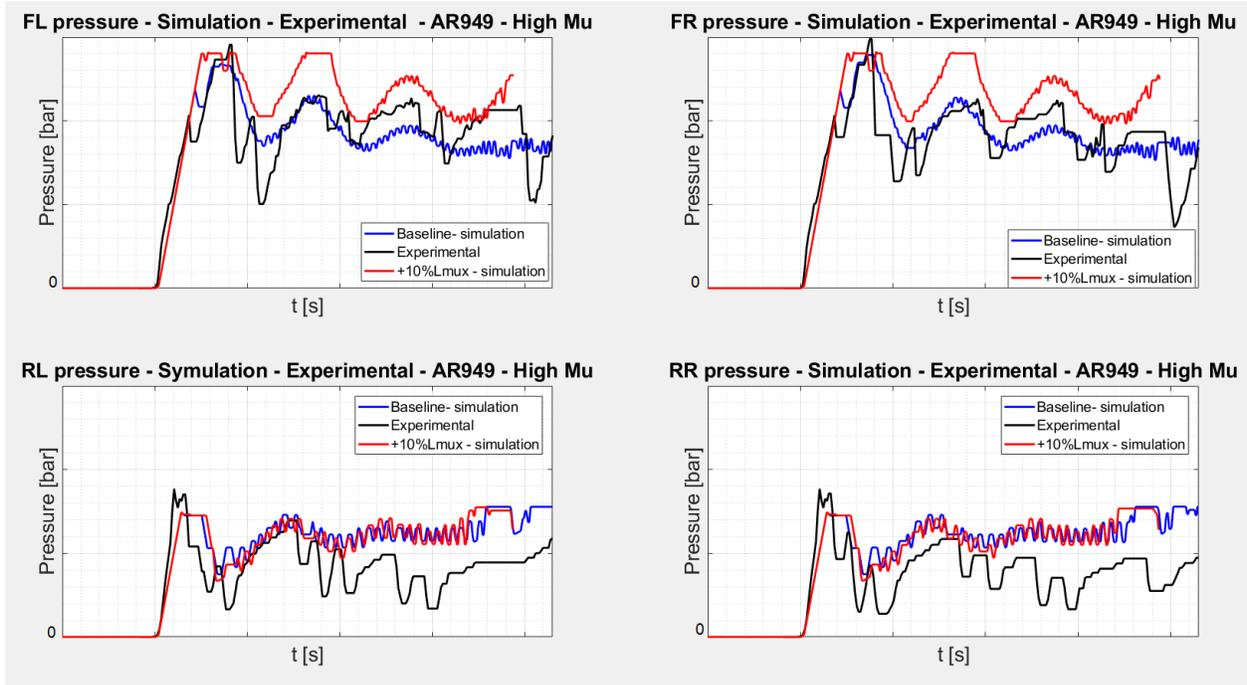
Figure 10.3.2 – Brake pressure on the four corners – Baseline vs +10%LMUX
