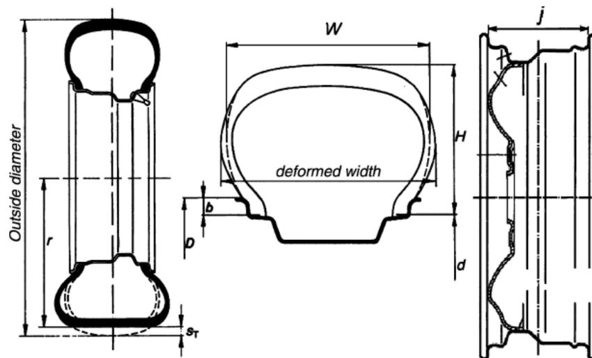
Figure 3.1 - Section of a complete wheel including rim and tire.
