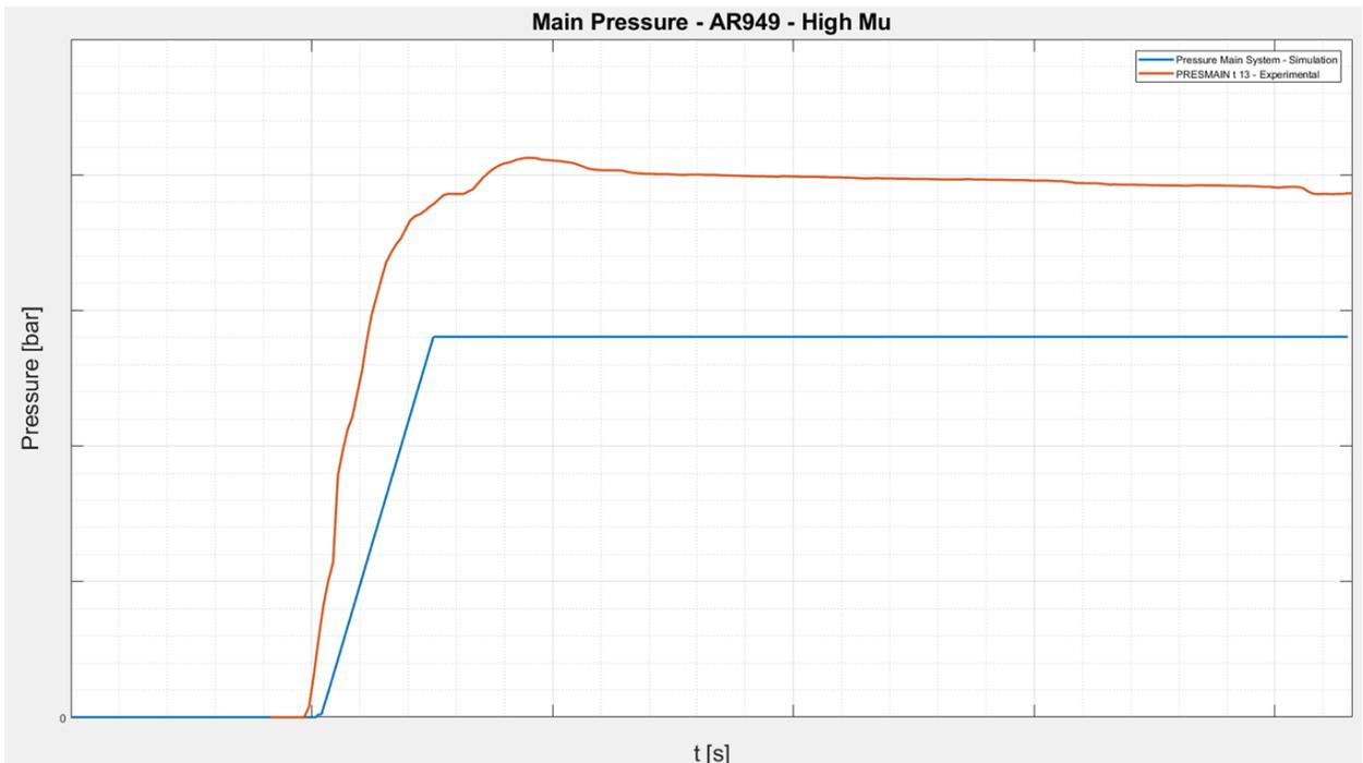
Figure 9.1.5 – Main System Pressure – AR949 on dry road
