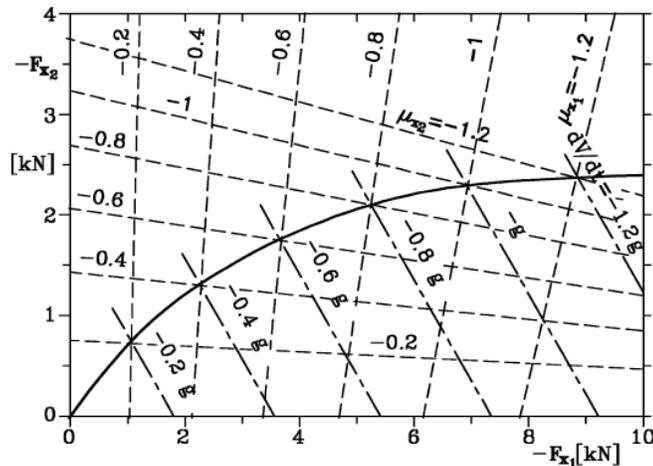
Figure 8.8 - Braking in ideal conditions. Relationship between  $F_{x_1}$  and  $F_{x_2}$
