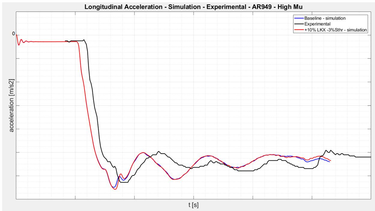
Figure 10.8.3 – Vehicle longitudinal acceleration – Baseline vs +10%LKX -3%Sthr
