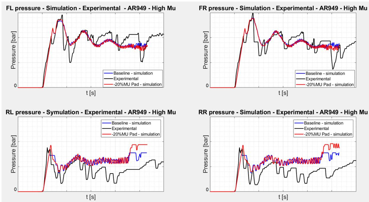
Figure 10.10.2 – Brake pressure on the four corners – Baseline vs -20% Pad's Mu
