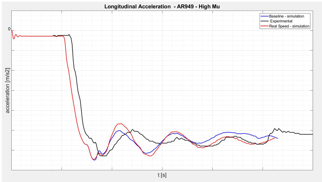
Figure 10.1.4 – Vehicle longitudinal acceleration – Baseline vs CRT real speed
