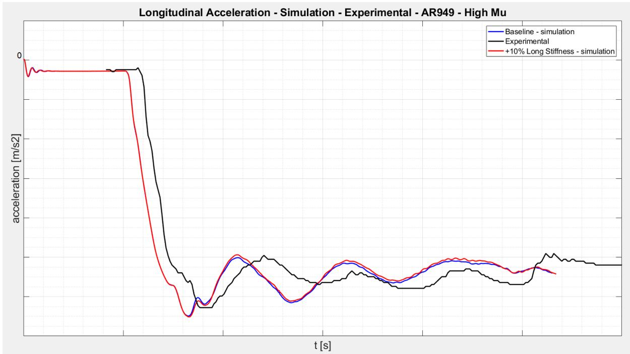
Figure 10.13.3 – Vehicle longitudinal acceleration – Baseline vs +10% Structural longitudinal stiffness
