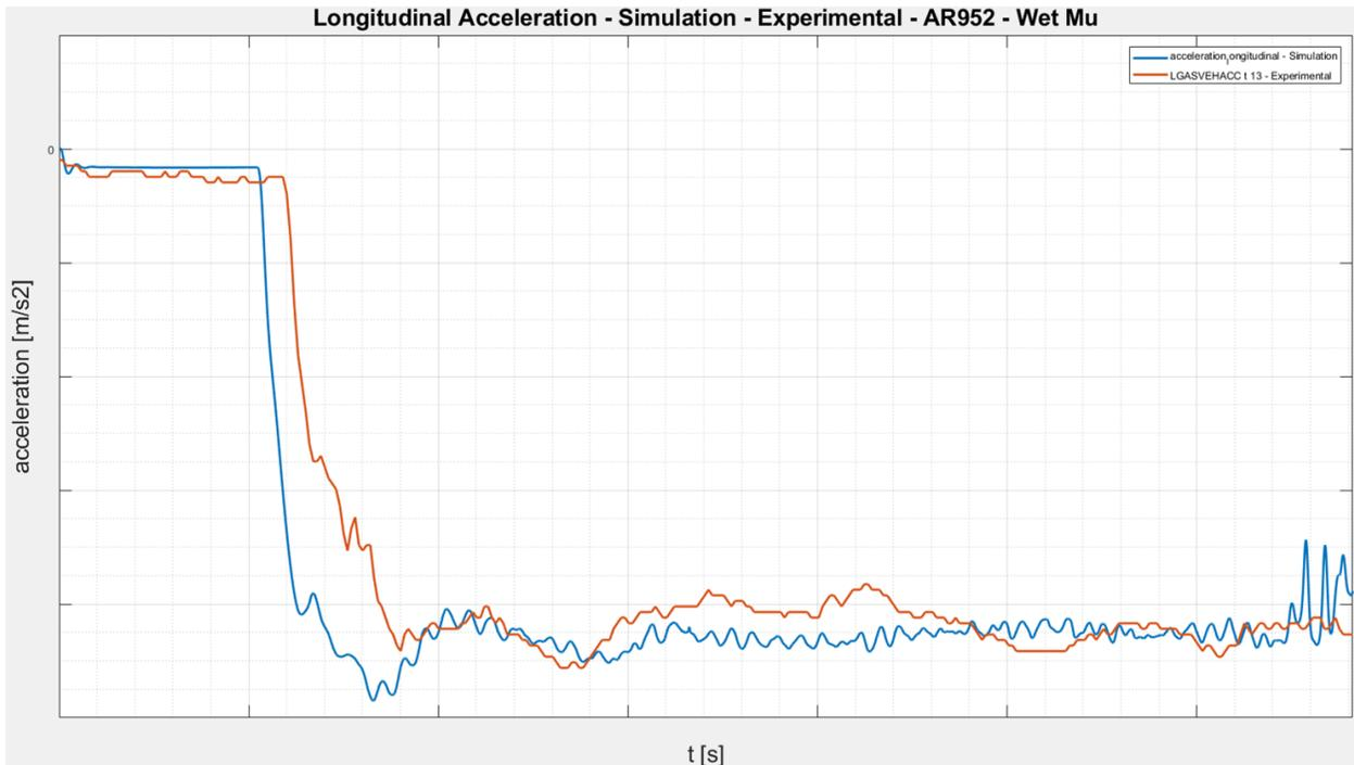
Figure 9.2.6 – Vehicle longitudinal acceleration – AR952 on wet road
