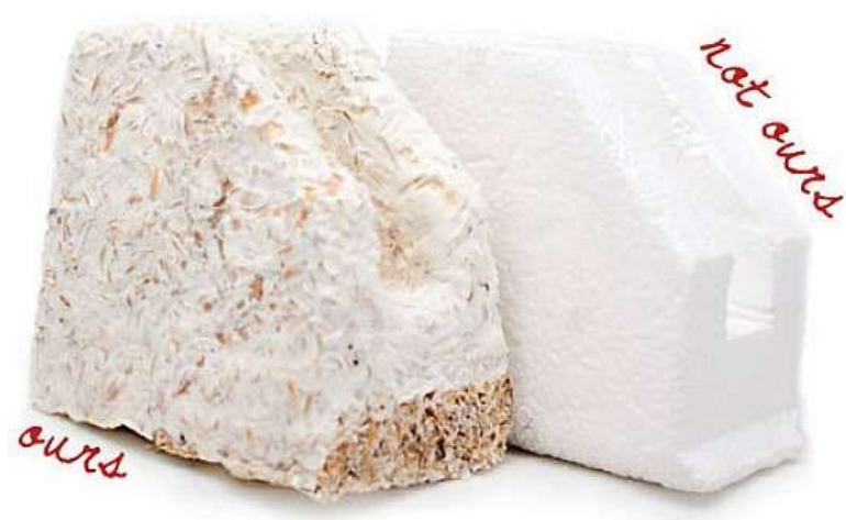
Figure 2: Unicel vs. Mycelium Material
