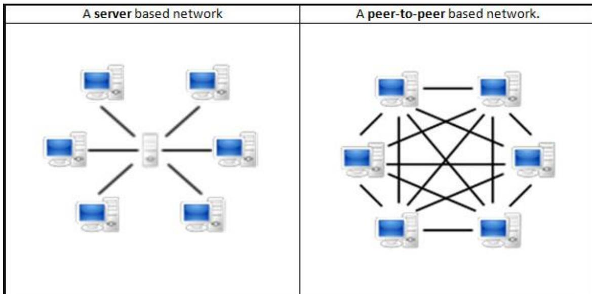
Figure 4 - Server based vs P2P based network (Source: Bitcoinwiki.org)
