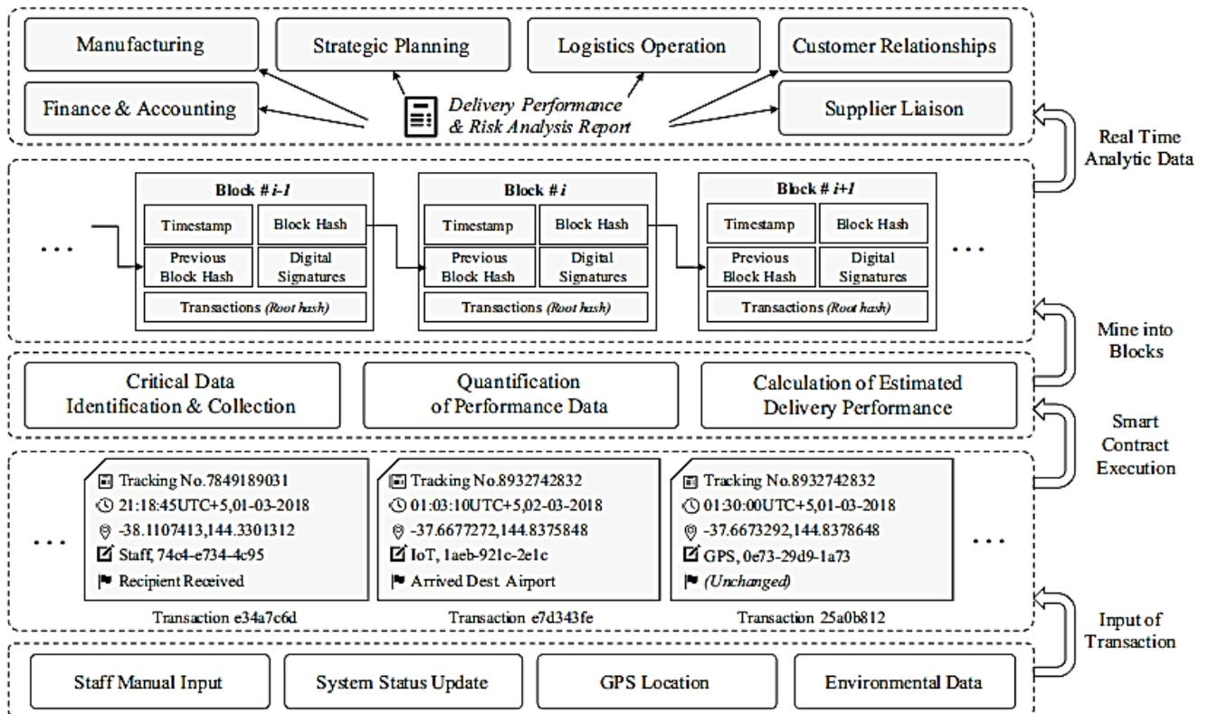
Figure 17 - Architecture of a Blockchain based Supply Chain system. (Source Meng & Qian, 2018)
