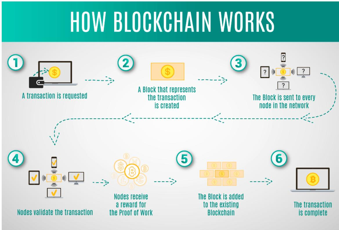
Figure 6 - How Blockchain works. (Source MLSDev.com)
