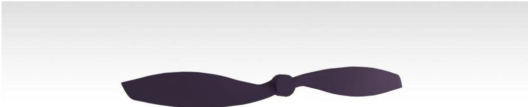
Figure 8.3: Rendered Image of the CAD model of the propeller APC 10x7 Slow flyer.
